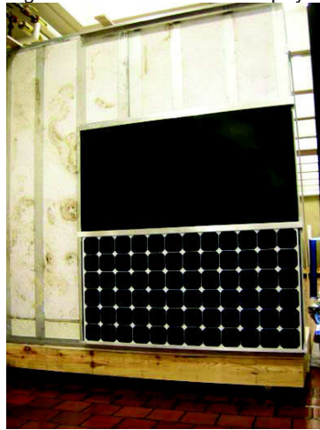
Figure 2: Full scale mock-up of PVs mounted on SIPs. Source: (Jamgochian 2006)
