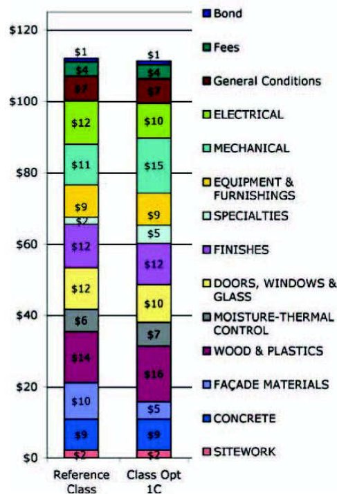
Figure 5: First cost comparison (per SF) between typical reference classroom and high performance classroom. (Source: BOORA Architects)
