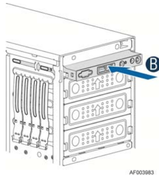
Figure 111. Installing the Front Panel Tray in Chassis
