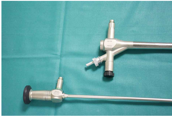
Figure 2. Adapter head of a Karl Storz (Tuttlingen, Germany) bronchoscope.
