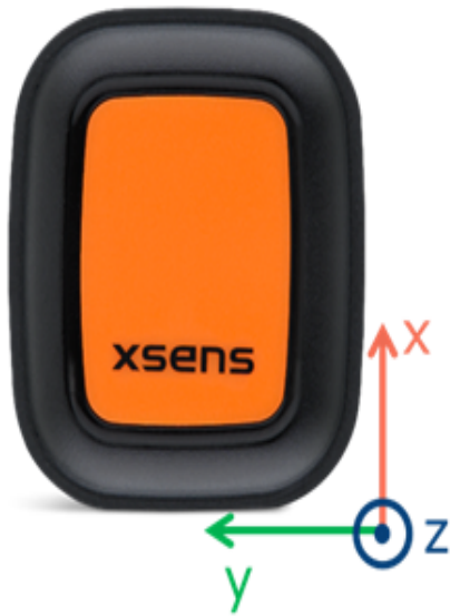
Fig. 22. The sensor frame of reference. The X axis is along the long edge, the Y axis along the short edge and the Z axis points outward.
