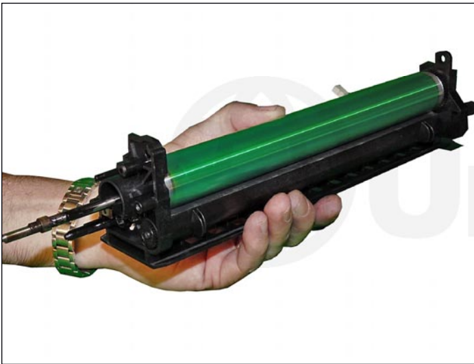
18. From the gear side, pull the drum axle out by grasping the axle.
