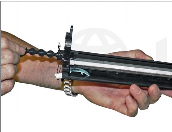
20. Remove the auger and clean it off.
