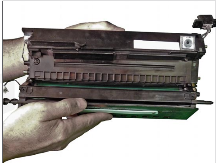
38. Align the drum/waste section pins so they fit into the supply hopper.
