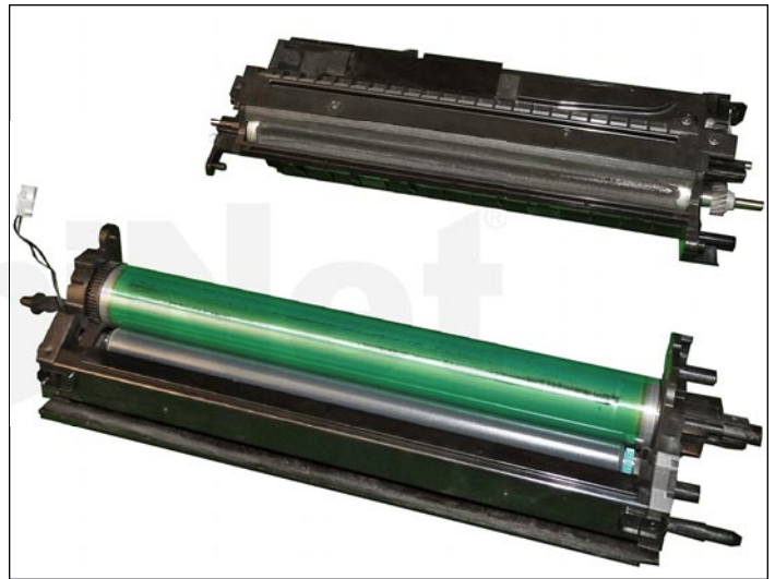
12. Separate the drum/waste hopper from the developer section.
