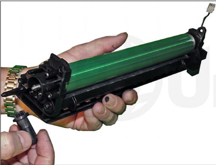
16. Remove the axle drive gear.
