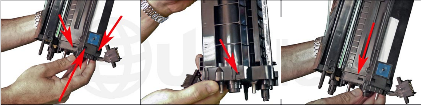
5. Press in on the four tabs and remove the lower end cap.
