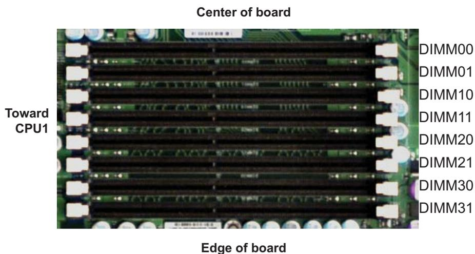
**Figure 5-8. Installing DIMM into Memory Slot**
