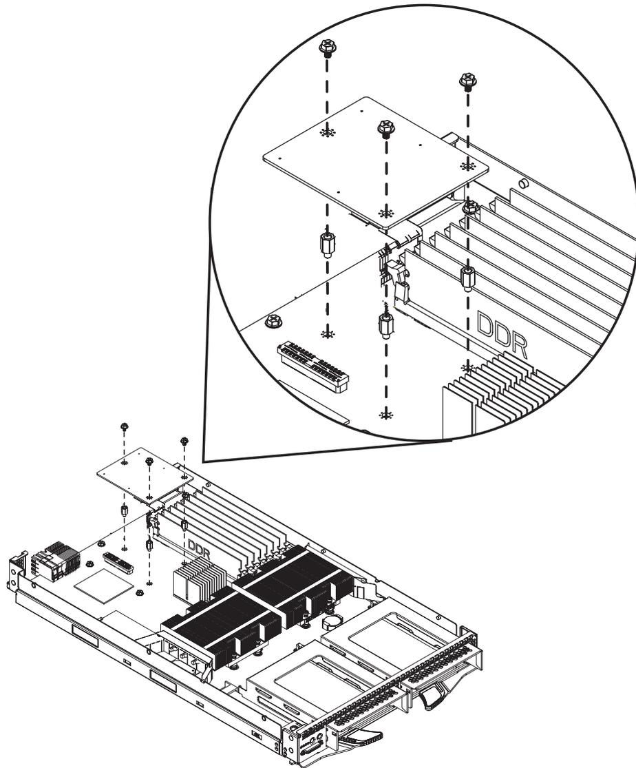
Figure D-3. Card Installation
