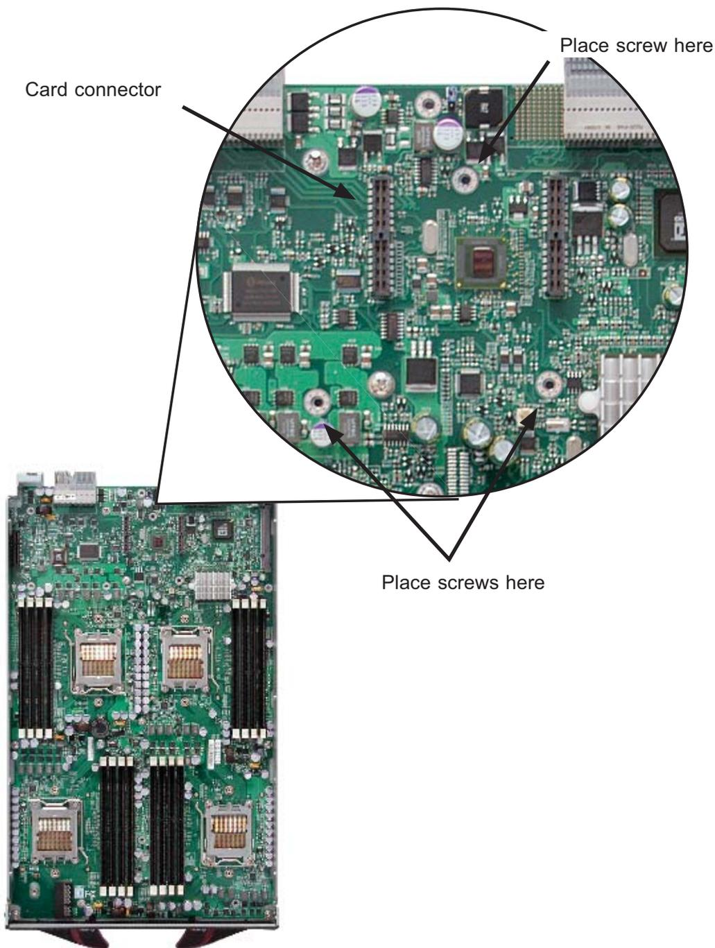
**Figure D-2. Installation Location**
