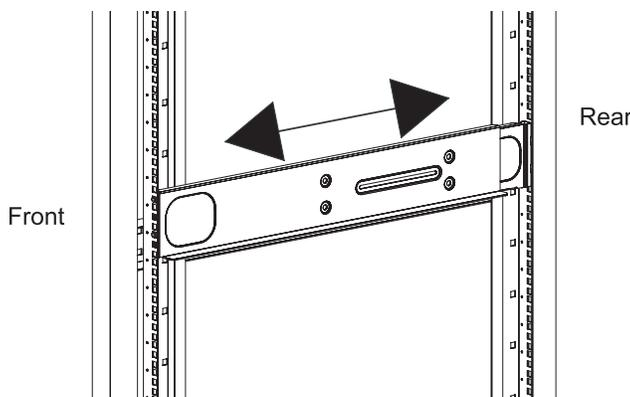
**Figure 3-3. Attaching the Optional Handles**
