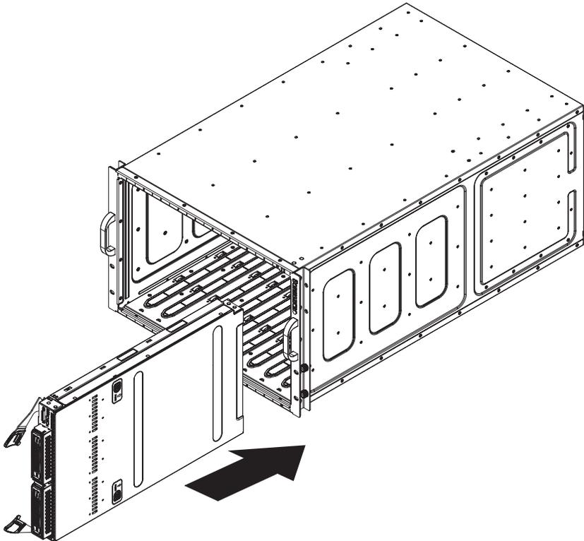
Figure 4-9. Locking the Blade into Position
