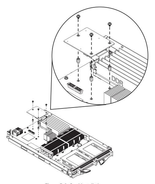
Figure D-3. Card Installation
