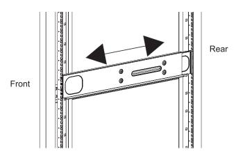
Figure 3-3. Attaching the Optional Handles
