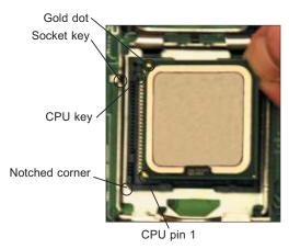
Figure 5-4. Installing a Processor in a Socket
