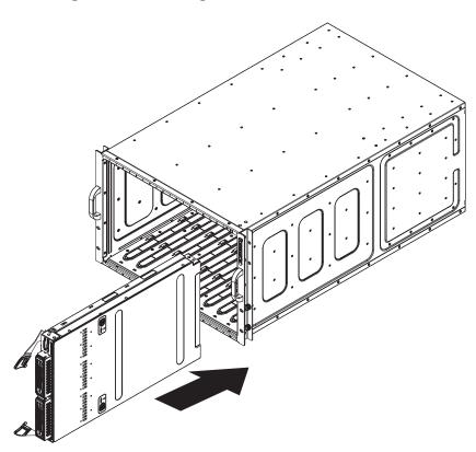
Figure 4-8. Inserting a Blade into the Enclosure
