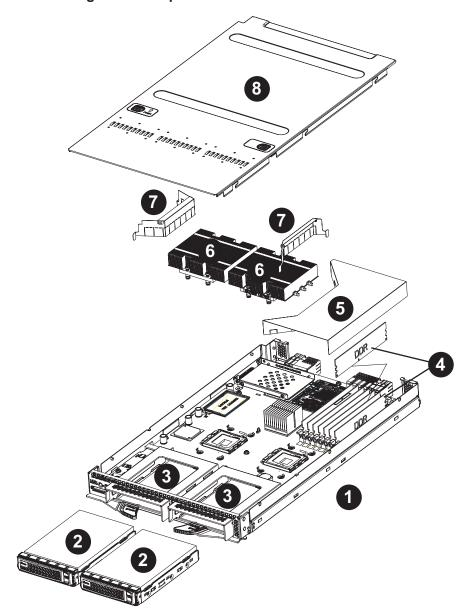
Figure 5-6. Exploded View of Blade Module
