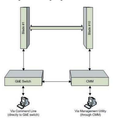
Figure 4-7. Configuring the GbE Switch
