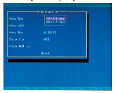
Figure 6-8. Array Assignment
