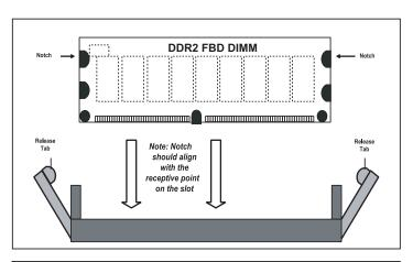
To Remove: Use your thumbs to gently push each release tab outward to free the DIMM from the slot.
