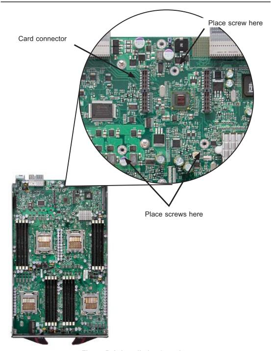
Figure D-2. Installation Location
