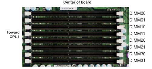
Figure 5-8. Installing DIMM into Memory Slot
