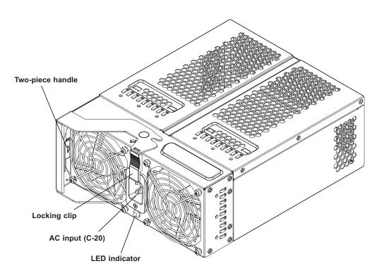
Figure 5-11. Power Supply Module
