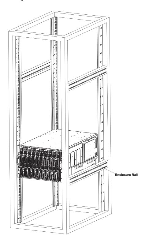
Figure 3-4. Enclosure Installed into Rack
