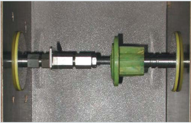
Figure 1: Wall bushing with formwork installation
