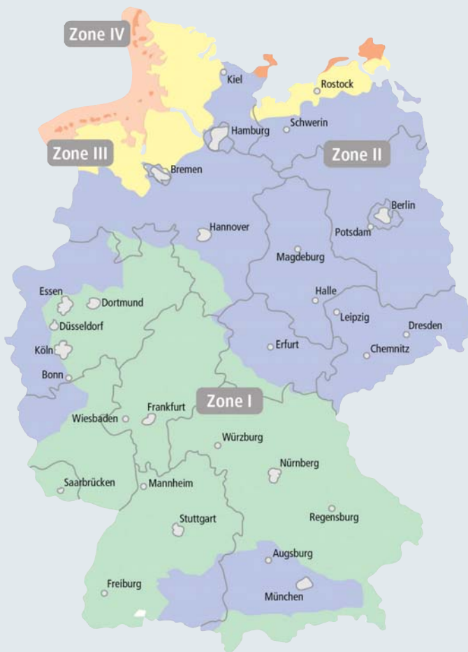
Figure 1: Wind load zones in Germany and corresponding values of dynamic pressure and maximum wind speed
