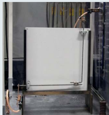
Figure 5: Specimen fixed on insulating plate (MV clamp) for a test in the impulse current laboratory
