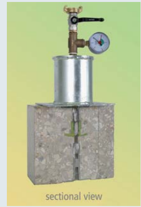
Figure 2: Set-up with terminal for the pressure-water test
