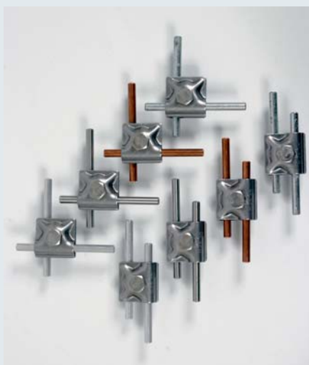
Figure 4: Test combinations for MV clamps (parallel and cross arrangement)
