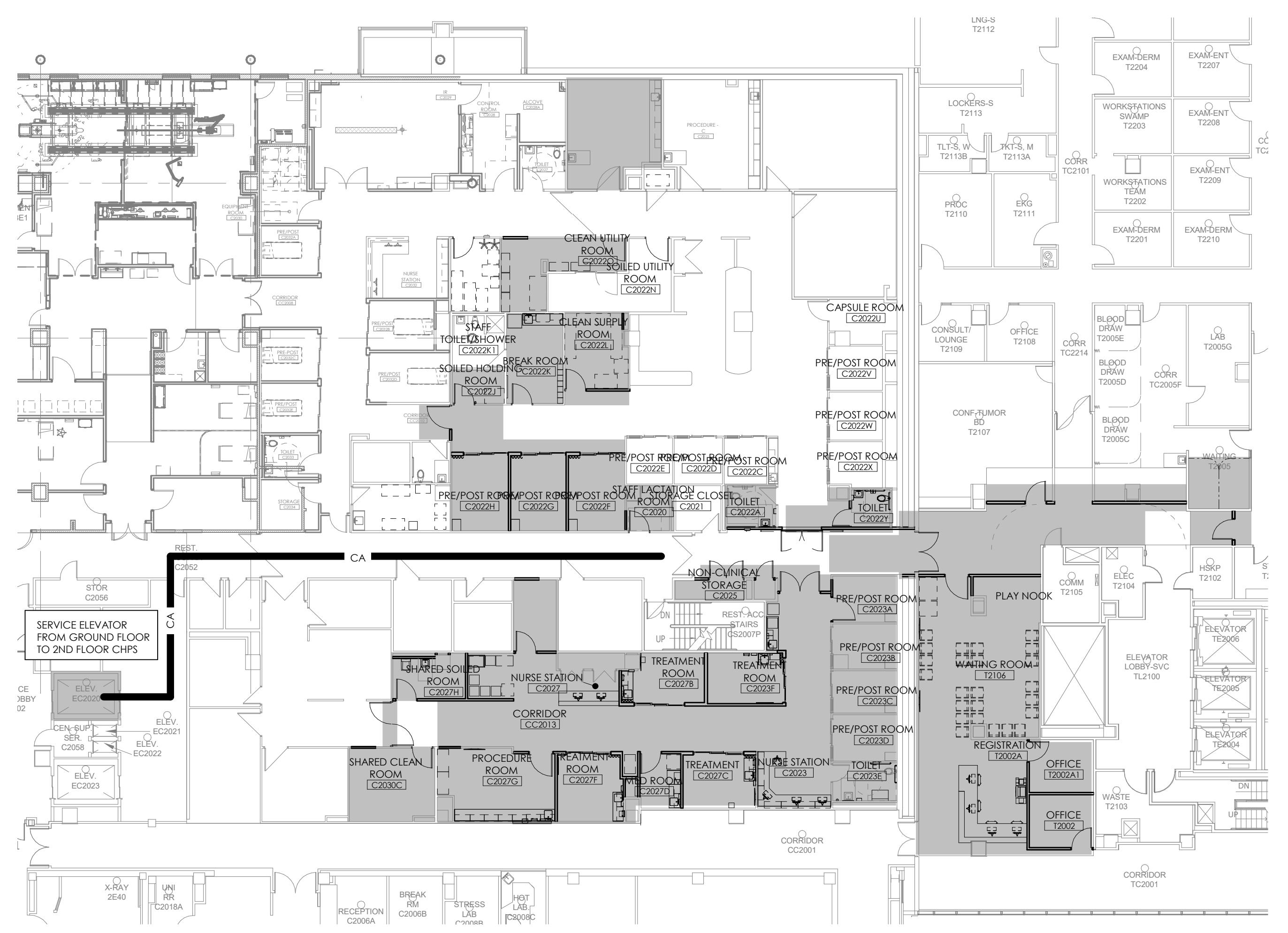
1 LEVEL 2 - CONTRACTOR ACCESS PLAN 1/16" = 1'-0"
