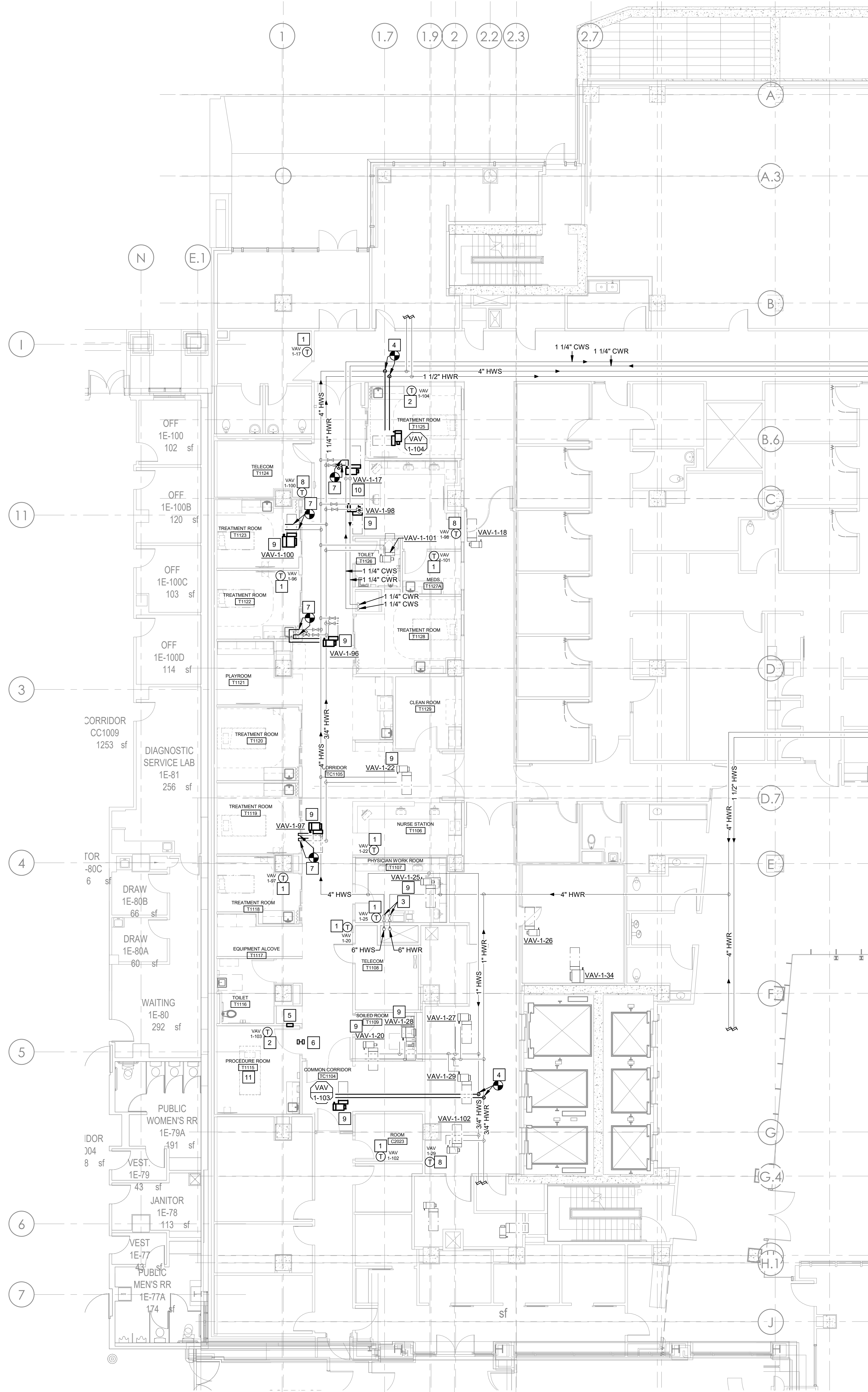
1 FIRST FLOOR CBCU - MECHANICAL PIPING - NEW WORK 1/8" = 1'-0"
