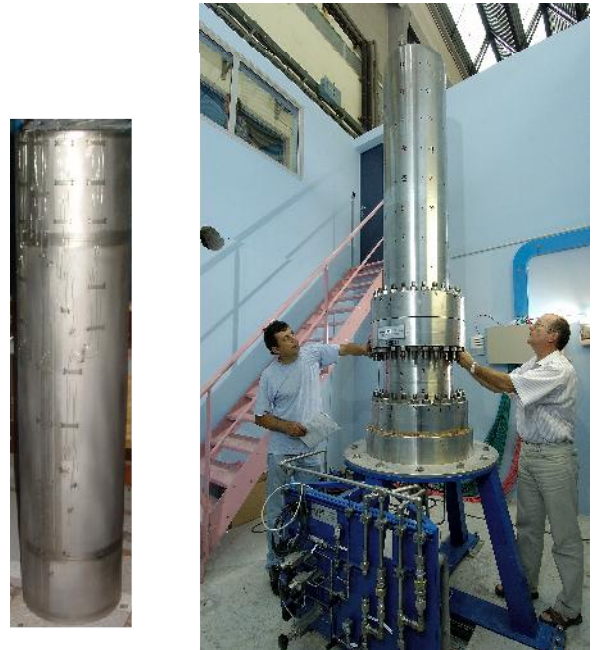
Figure 1: On the left view of the "Encapsulated" concept thermal barrier – On the right the HETHIMO facility
