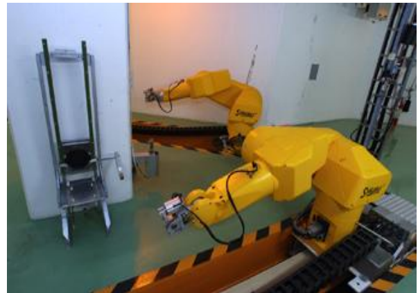
Figure 9: Stäubli RX robots used at the Isolde facility
