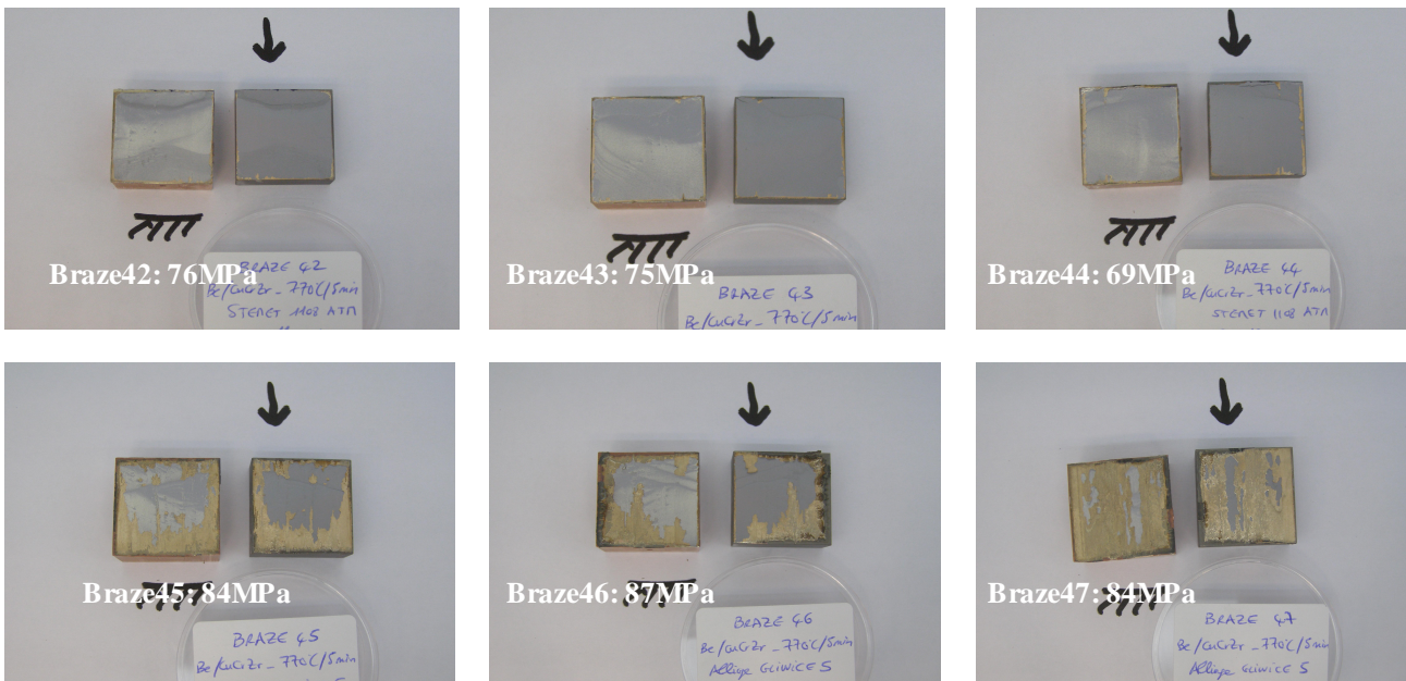
Figure 4: Views of brazed samples after shear tests
