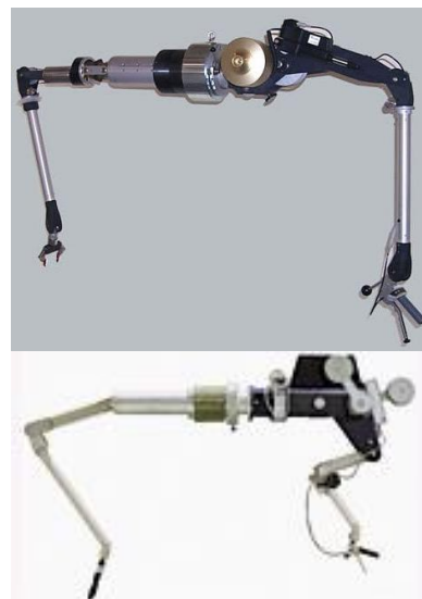
Figure 2: Example of articulated manipulator (MA11 La Calhène, A200 Wälischmiller)
