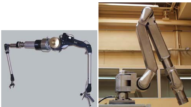
Figure 1: MSM and Manipulator t examples with six rotational joints in series
