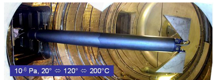
Figure 1: Test campaign on the ITER relevant module under real functioning conditions (February 2007)
