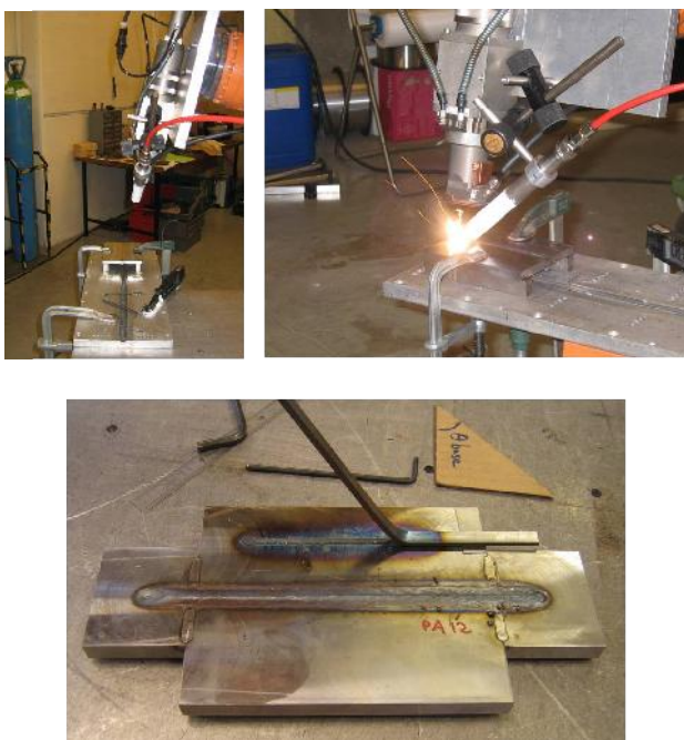
Figure 5: Eurofer 11mm thickness samples welding
