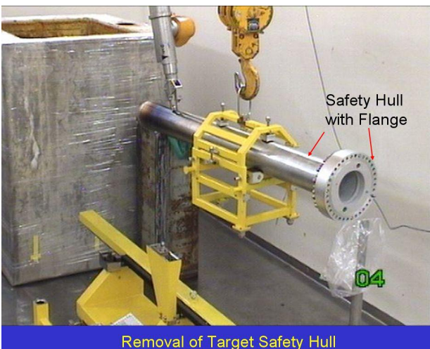
Figure 8: Operations in hot cell on SINQ target
