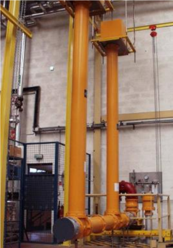
Figure 2: Several RF tests of components including dedicated mock-ups and full-size prototypes pieces of the ITER IC antenna will be required within the framework of the R&D program. Upgrading of existing test facilities has been proposed to fulfil ITER IC antenna testing programme. Figure 2 show the Tore Supra RF test stand facility. This existing installation is presently limited to the test of components water cooled at low temperature (chilled water below 35°C). Regarding the ITER operating conditions in term of cooling, an upgrade of the test stand is necessary to test water RF components within the ITER specification for the water cooling (100 à 150°C / 20 à 40bars)
