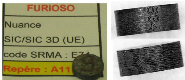
Figure 3: Specimen markings, on left traces of felt pen marking on diffusivity specimens, on right laser marking
