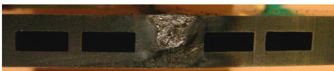
Figure 1: Cooling plates mock-up after welding
