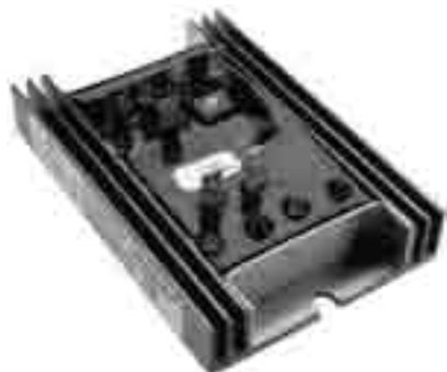
V1300 Regulator 12 Volt, B-Circuit, 14.2 Vset
