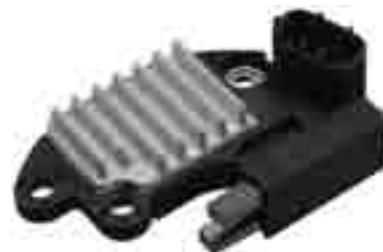
D1621 Regulator / Brush Holder Assy. 12 Volt, A-Circuit, S-IG-L Terminals, 14.4 Vset, 5 sec. LRC
