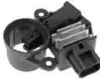
F600 (Ref# 35-212) Regulator / Brush Holder Assy. 12 Volt, A-Circuit, I-D-A Terminals 14.4 Vset, wo/ LRC, Gray w/ Gray Cover
