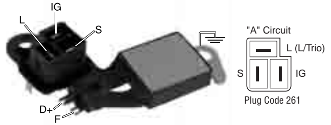
IN229 (Ref# 35-8202) Regulator 12 Volt, A-Circuit, L-S-IG Terminals, 14.1 Vset
