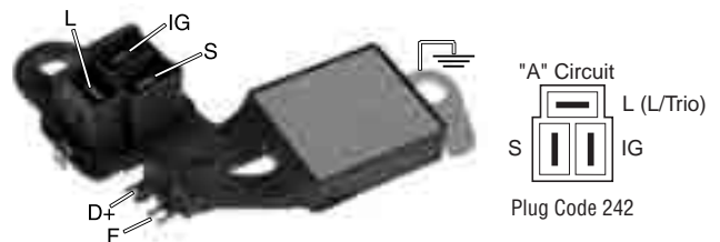
IN230 (Ref# 35-8222) Regulator 12 Volt, A-Circuit, L-S-IG Terminals, 14.1 Vset
