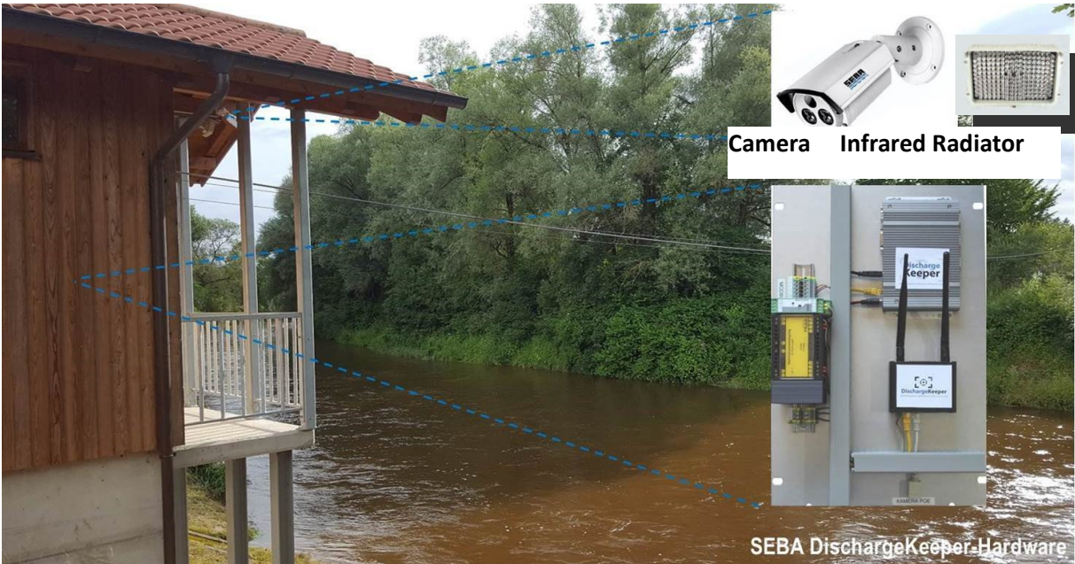
Figure 1: Hardware components of the DischargeKeeper for a typical measuring site
