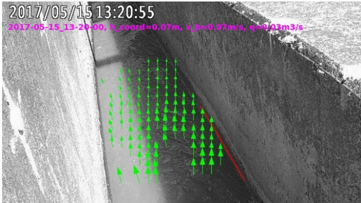
Figure 9: DischargeKeeper's measuring site on the inflow of a waste water plant
