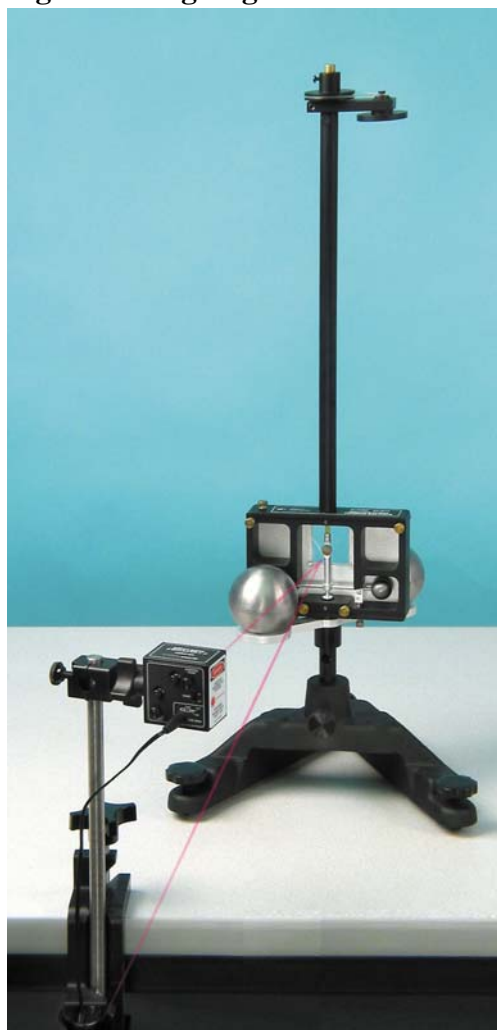
Figure 7b: Setting up the Optical Level
