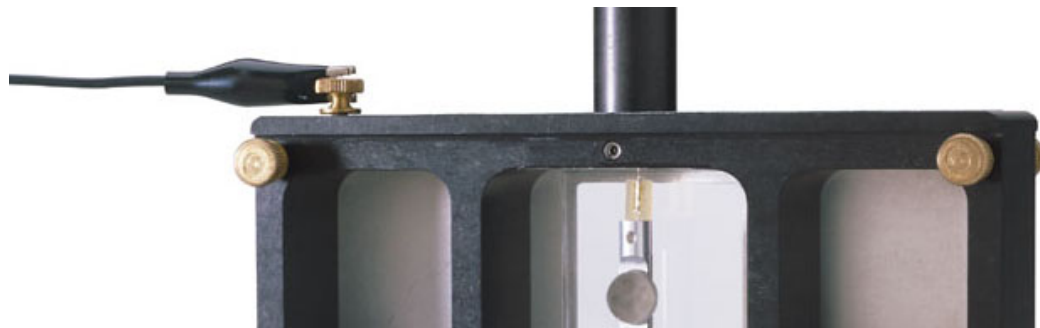
Figure 10: Attaching the Grounding Strap to the Grounding Screw
