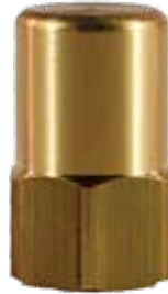
SE-RCAP-01B Material: Brass Height: 1-3/8" Thread: 3/4"-16 505-0431-00
