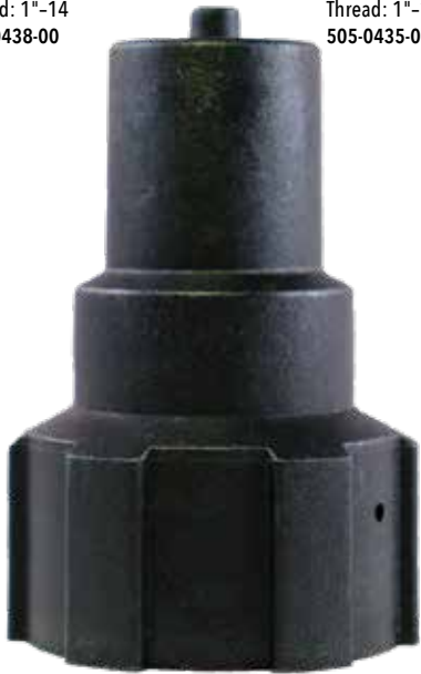
SE-RCAP-08P Material: Valox Height: 3-1/8" Thread: 1-5/8"-12 005-0664-00
