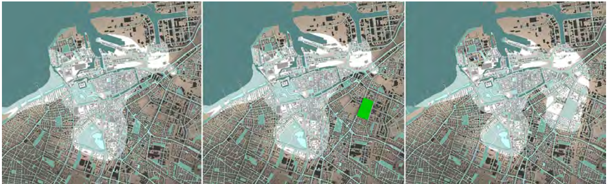
Figure 5. A new area is drawn in green as a polygon in the Map Viewport. This area is then added to the loaded park data which directly changes the fitness function and the white field showing the area with highest fitness.
