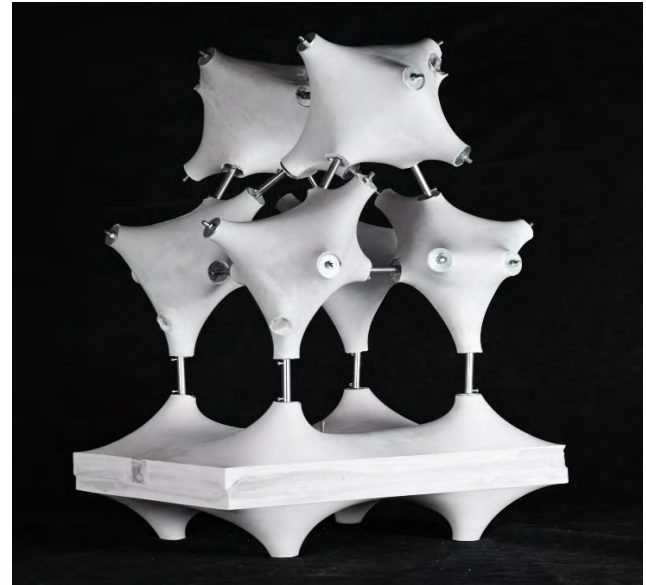
Figure 10. The resulting demonstrator with hollow body concrete nodal component.
