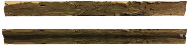
Figure 1. Samples for structural tests of Concrete and of PET in Concrete as a gradient
