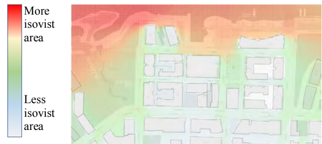
Figure 2. Isovist area of visible space 1 . The area of visible space from each cell. Proportional to the number of cells directly visible from each cell.
