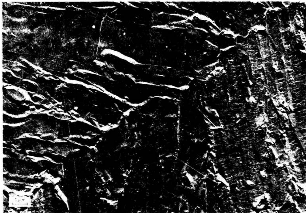
Figure 4.3.2-9 — Microstructure of CVD Silicon Carbide at Joint of Two Adjacent Areas (7100X)
