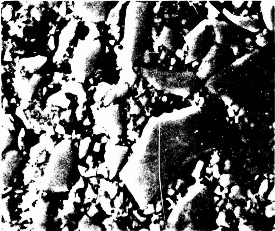
Figure 3.2.2-3 — Microstructure of Cast Silicon Structure (800x)
