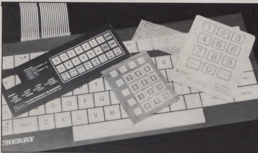
Photo 1. Various membrane panels that are available. The one shown from Cherry Electric (Waukegan, IL) is a full ASCII keyboard with tactile feel.
