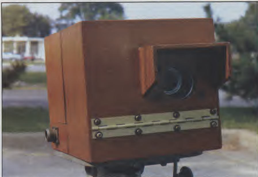
Front view of meteor camera in environment enclosure.
