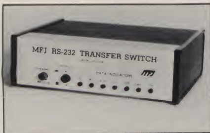
The MFJ RS-232 Transfer Switch switches between two RS-232 devices and presents a visual display of the status of the individual signaling lines. The unit can also swap lines 2 and 3 with a push of a button.
