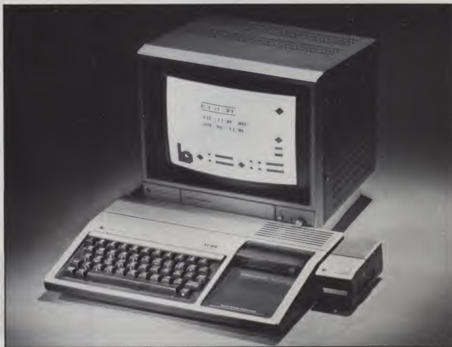
The TI 99/4A was the first home computer console to offer a 16-bit central processing unit. With the machine's language, TI Basic, 16 colors can be programmed for graphic effects; music and sound effects also can be generated.
