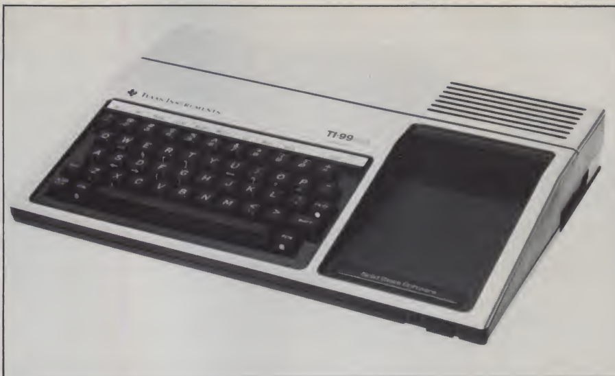
Encased in a brush-aluminum console with black plastic trim, the TI 99/4A features a 48-key keyboard and upper- and lowercase letters.
