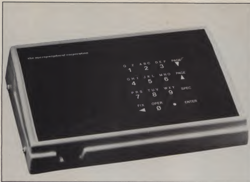
The Bank Box remote banking terminal from the Microperipheral Corporation can receive graphic images from a host system at 1200 baud. It is designed to sell in quantity for less than $100.
