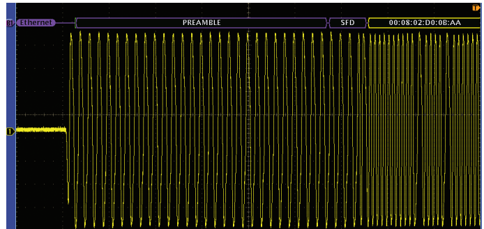
Figure 7. Ethernet Preamble (PRE) and Start-of-frame Delimiter (SFD).
