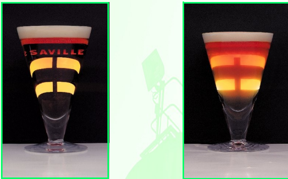
Presentation spoilt by the development of permanent post filtration haze due to high tannin (polyphenol) / protein content prior to (left) and following forced storage.
