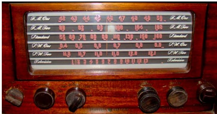
Dial of the GE 901 showing the old FM One and newly allocated FM Two bands, as well as AM and Short Wave bands, and television channels 1-13.
