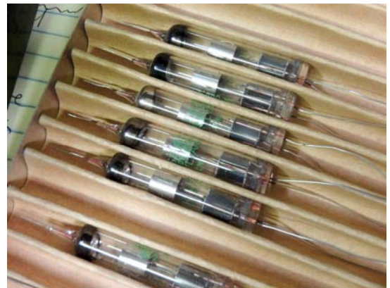
Miniature vacuum tubes used as a substitute for high voltage vacuum capacitors.
