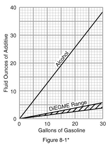
Prolonged storage of the airplane will result in a water buildup in the fuel which leeches out the additive. An indication of this is when an excessive amount of water accumulates in the fuel tank sumps. The concentration can be checked using a differential refractometer. It is imperative that the technical manual for the differential refractometer be followed explicitly when checking the additive concentration.
