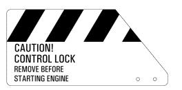
3. Silk-screened on left instrument panel above magnetos switch:
