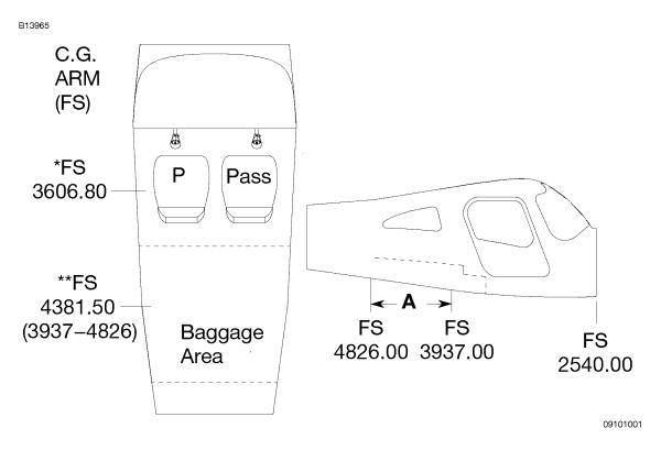
\*Pilot and front seat passenger center of gravity for average occupant.
