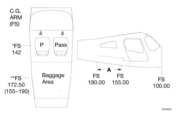
\*Pilot and front seat passenger center of gravity for average occupant.
