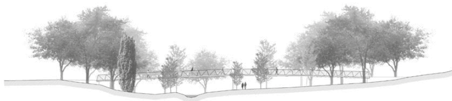
Figure 10. The proposed transversal section of the park. This area will work as a retention basin, accumulating a large volume of water
