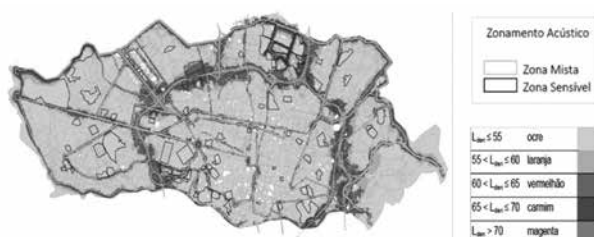
Figure 11. Adapted from the Noise Map of the city of Oporto, dated 07/31/2014, related to the L_{den} indicator (CMPorto, 2014)
