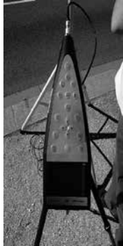
Figure 7. B & K sound level meter used for field measurements.
