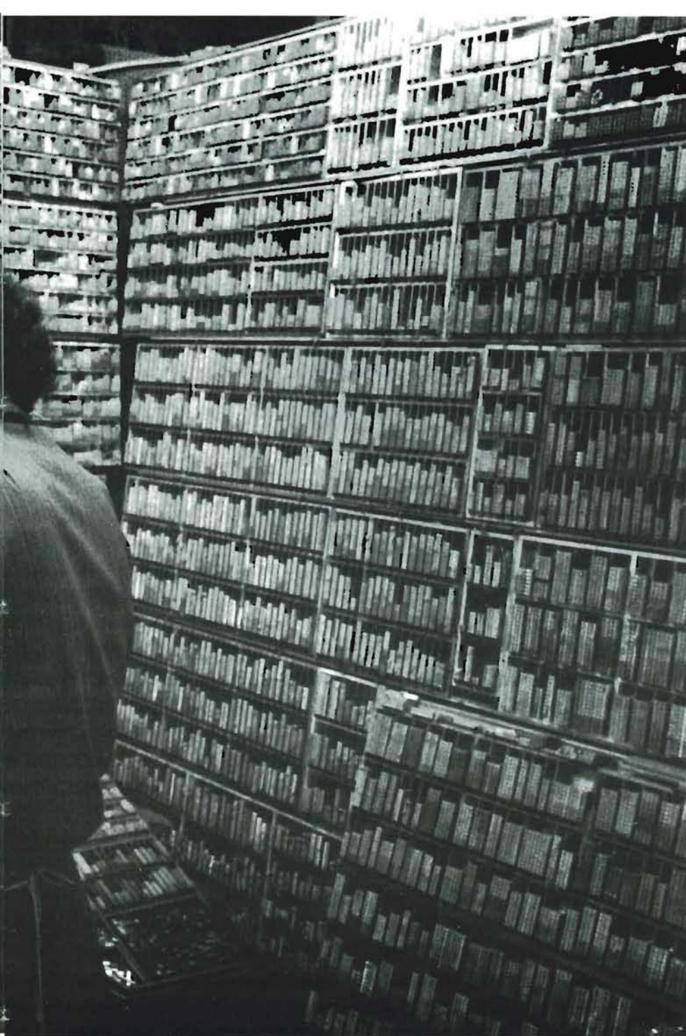
Hand setting the 6.3m daily run People's Daily newspaper from a 3500 character set. Speeds of 1000 characters are achieved an hour – equivalent to 3000 Latin language characters. (Photo : Bruno Barbier).
