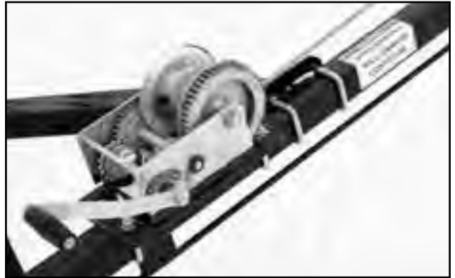
Fig 14 - Tube Lift Winch
