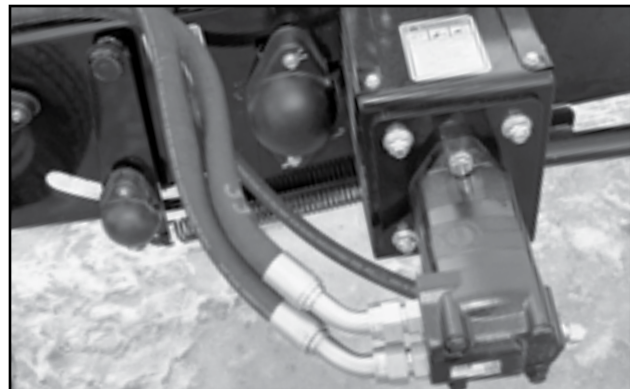
Fig 105 - Hydraulic Drive, Main Conveyor
