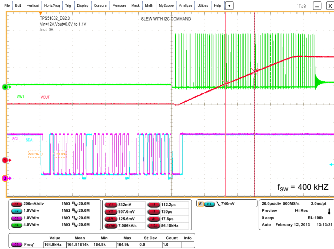
Figure 22. Startup at 400-kHz I 2 C Clock Speed
