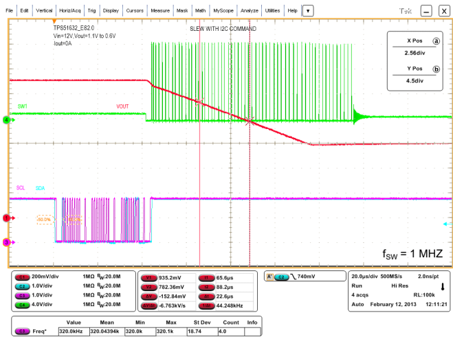
Figure 24. Startup at 1-MHz I 2 C Clock Speed
