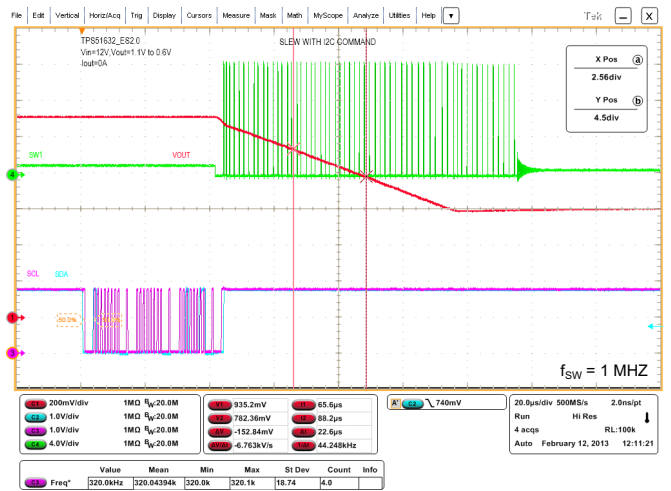
Figure 25. Shutdown 1-MHz I 2 C Clock Speed
