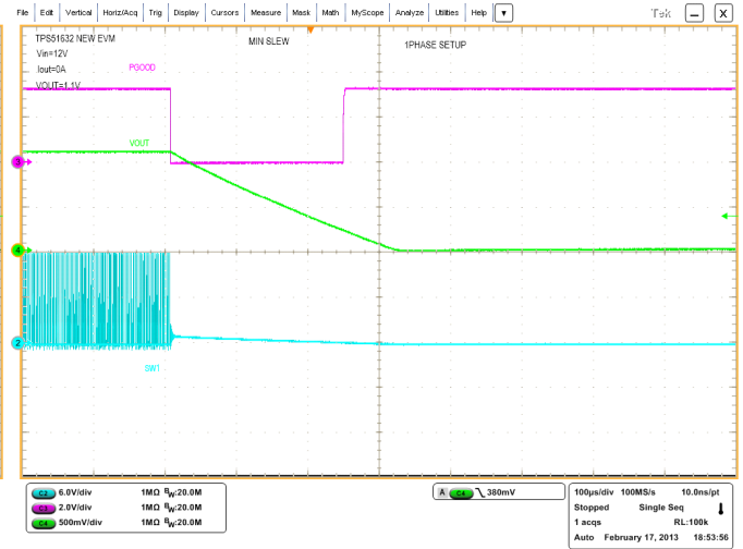
Figure 19. 1-Phase EN Shutdown
