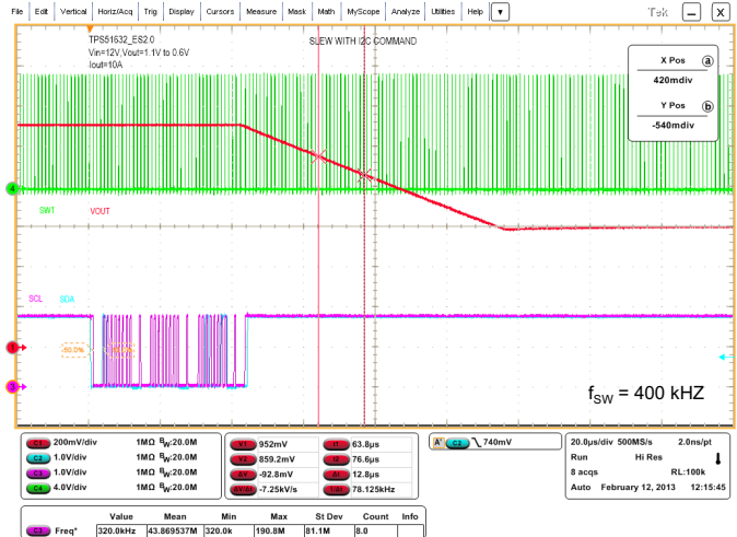
Figure 29. Shutdown 1-MHz I 2 C Clock Speed
