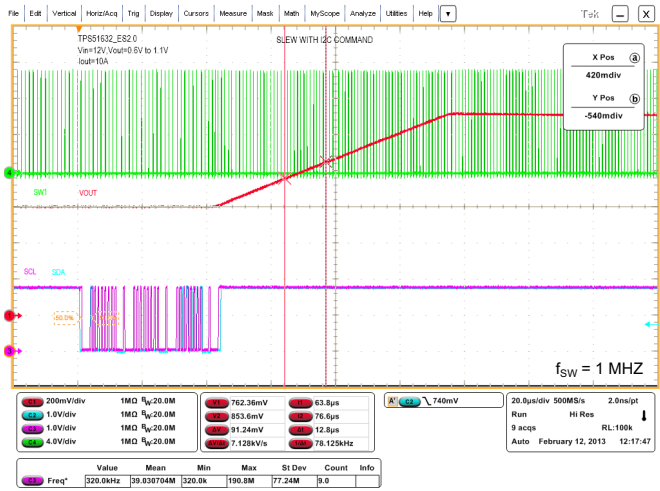
Figure 28. Startup at 1-MHz I 2 C Clock Speed
