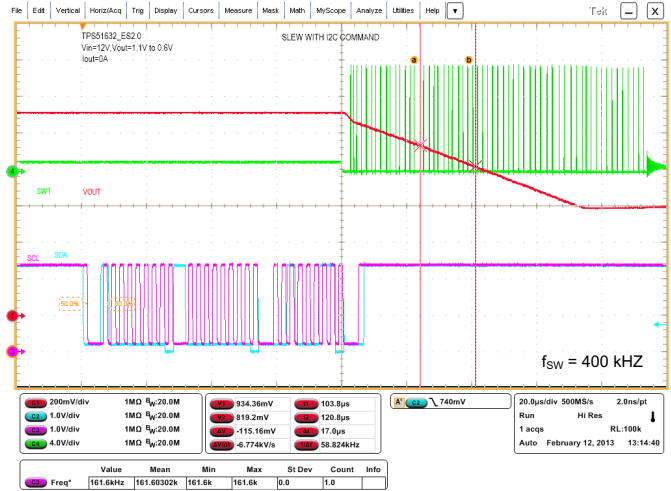
Figure 23. Shutdown 400-kHz I 2 C Clock Speed
