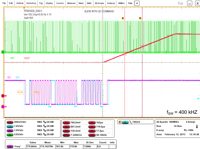
Figure 26. Startup at 400-kHz I 2 C Clock Speed
