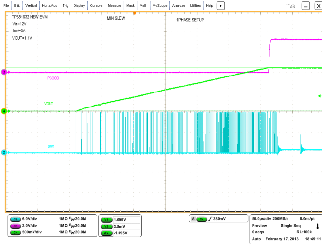
Figure 18. 1-Phase EN Startup
