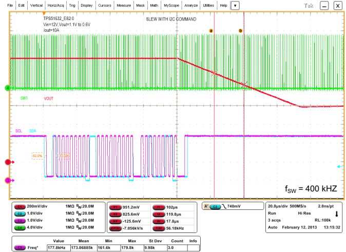
Figure 27. Shutdown 400-kHz I 2 C Clock Speed
