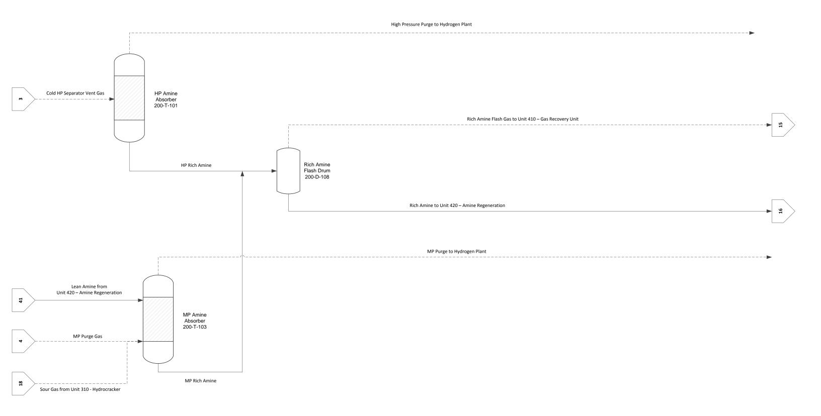
Domestic Synthetic Fuels I Process Flow Diagram Unit 310 – Hydrocracker
