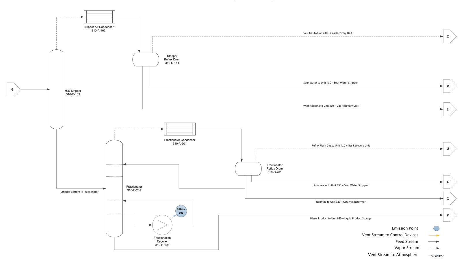
Domestic Synthetic Fuels I Process Flow Diagram Unit 320 – Catalytic Reformer
