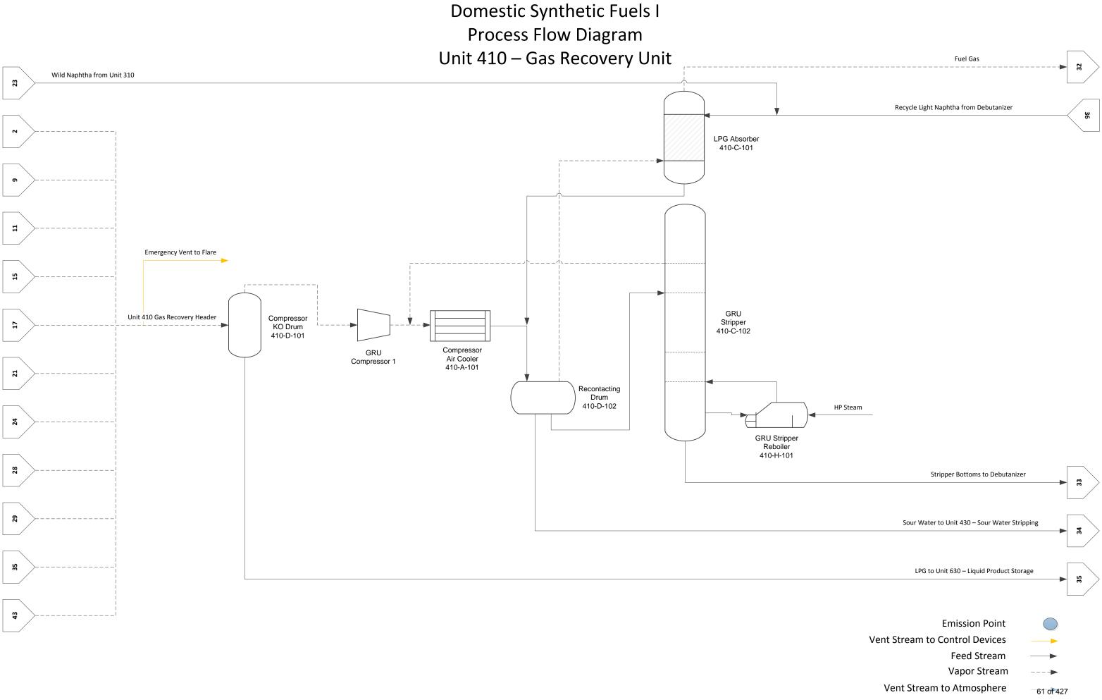
Domestic Synthetic Fuels I Process Flow Diagram Unit 410 – Gas Recovery Unit
