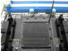
STEP 1: Lift Up The Socket Lever
