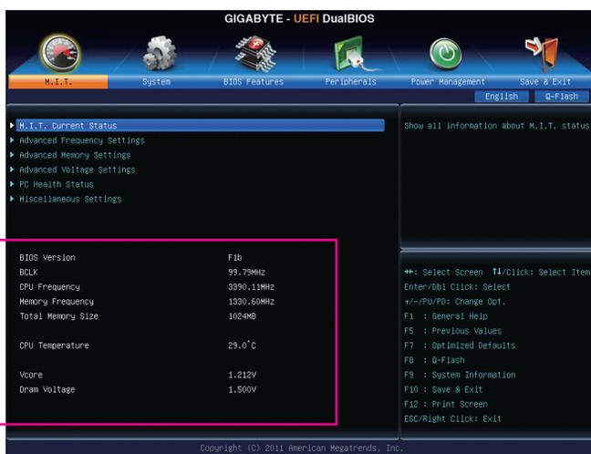
This section provides information on the BIOS version, CPU base clock, CPU frequency, memory frequency, total memory size, CPU temperature, Vcore, and memory voltages.
