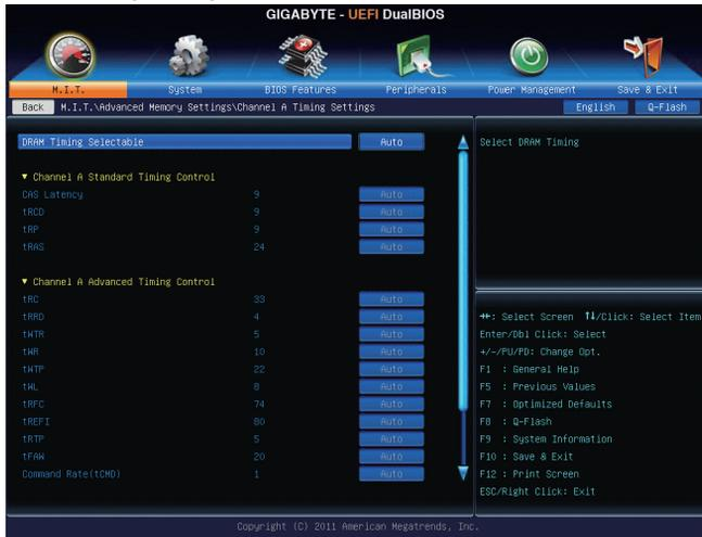
This sub-menu provides memory timing settings for each channel of memory. The respective timing setting screens are configurable only when **DRAM Timing Selectable** is set to **Quick** or **Expert**. Note: Your system may become unstable or fail to boot after you make changes on the memory timings. If this occurs, please reset the board to default values by loading optimized defaults or clearing the CMOS values.
