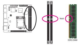
A DDR3 memory module has a notch, so it can only fit in one direction. Follow the steps below to correctly install your memory modules in the memory sockets.
