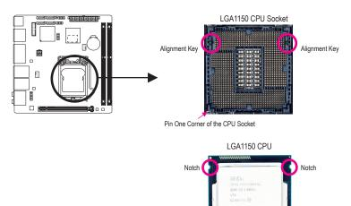
Triangle Pin One Marking on the CPU
