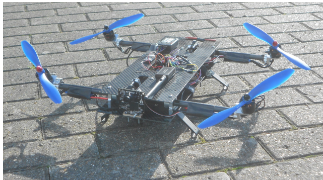
Fig. 1. Manufactured Prototype of a QTR used for flight tests
