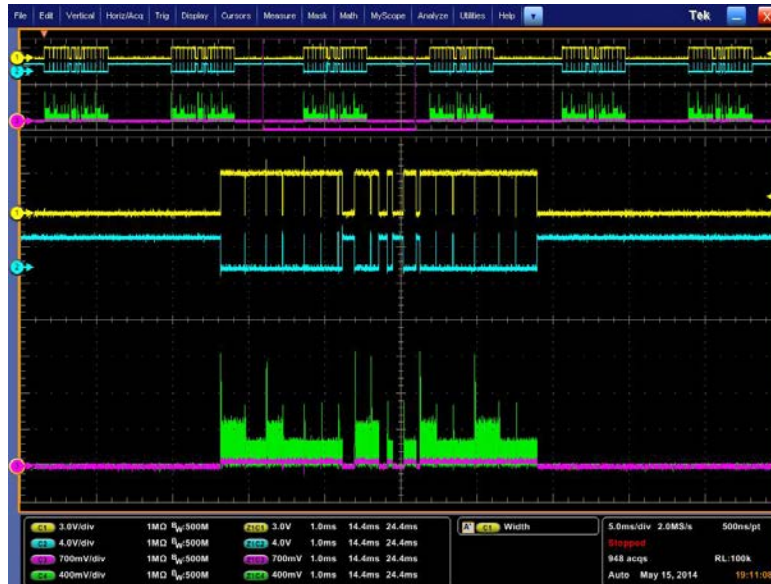
Figure 20: Continuous Mode: Normal operation in LDC2 with low PWM
