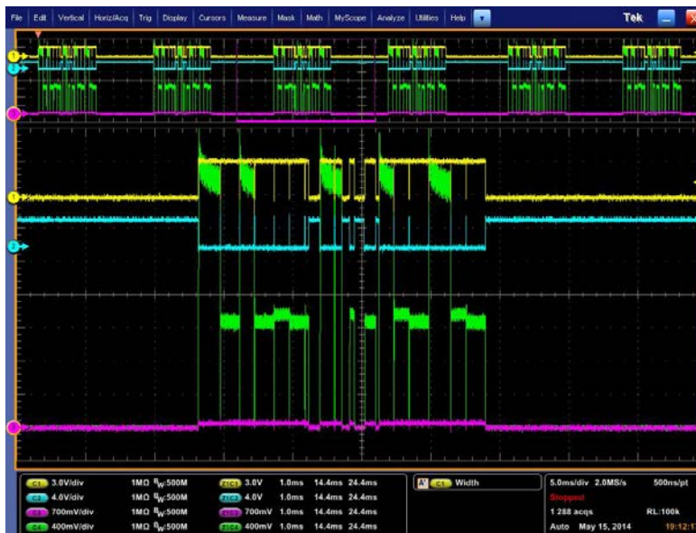
Figure 21: Continuous Mode: LDC2 photodiode fails open
