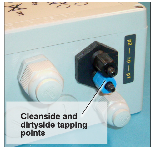
Figure 5 \Delta P connections
