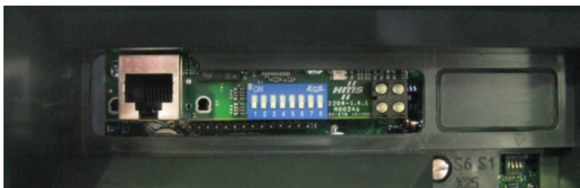
Figure 3-9 Modbus TCP board
