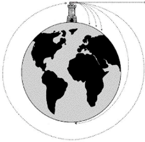
Illustration showing that if a cannon ball were shot fast enough, it would go around the Earth.
