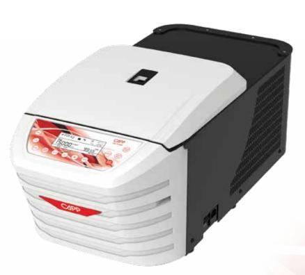
With four interchangeable rotor options the CAPP Rondo 44-place Refrigerated Centrifuge can handle a broad range of centrifugation tasks. The 44-place (22388 x g) and 24-place (21420 x g) rotor options accommodate 1.5mL and 2mL microcentrifuge tubes. Larger 5mL microcentrifuge tubes can be spun using the 8-place (18462 x g) rotor. Additionally, it can accommodate PCR strips in a special PCR strip rotor (15397 x g).
