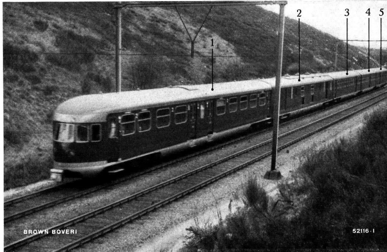
Fig. 1. — Diesel-electric 5-coach train, 1950 H. P. belonging to the Dutch Railways. 1, 3, 4 and 5 = passenger coaches. 2 = engine coach.
