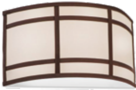
WF-K177-115-01-506OB ADA Sconce Finish: Oil Rubbed Bronze Fabric: White Linen with 1/2" Chocolate Silk Trim Length: 8" • Width: 15" • Depth: 4" Backplate: 10" x 6" Shade: (15" x 4") x (15"x 4") x 8" 2 – 60 Watt Max Candelabra Bulbs
