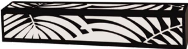
WF-STCUS-LCM-926P-MBK ADA Wall Fixture–Finish: Matte Black Material: Laser Cut Steel/Opal Acrylic Length: 18"• Width: 4"• Depth: 2 1/2" Canopy: 18" L x 4" W Shade: (4" x 2 1/2") x (4" x 2 1/2") x 18" H LED: Available in 3000K, 3500K and 4000K
