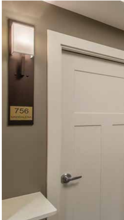
WF-CUS3-115-01-SN ADA Name Plate Sconce Finish: Satin Nickel Shade Material: White Butcher Linen Length: 30" • Width: 5 3/4" • Depth: 4" Backplate: 30" x 5 3/4" Shade: (4 1/2" x 3 1/2") x (4 1/2" x 3 1/2") x 8" Engraved Plate: 5" L x 4" H 1 - Candelabra Based
