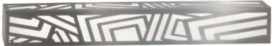
WF-STCUS-LCM-928M-SVPC ADA Wall Fixture – Finish: Silver Powder Coat Material: Laser Cut Steel/Opal Acrylic Length: 32" Width: 4" Depth: 2 1/2" Canopy: 32" L x 4" W Shade: (4" x 2 1/2") x (4" x 2 1/2") x 32" H LED: Available in 3000K, 3500K and 4000K
