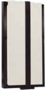
WF-12X6ST-115-01-PR-OB Providence ADA Sconce Finish: Oil Rubbed Bronze Shade Material: White Butcher Linen Length: 12" • Width: 6" Depth: 4" Backplate: 12" L x 6" w x 2" D Shade: (5.75" x 3.75") x (5.75" x 3.75") x 11 5/8" H 2 – Candelabra Based
