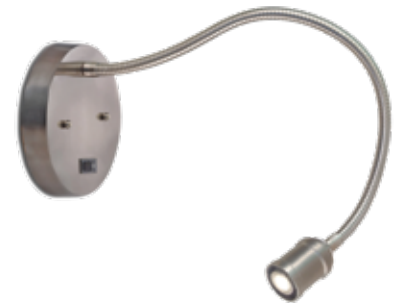
WF-A099-LED-SN LED Reading Light with Flexible Shaft Finish: Satin Nickel Length: 5 1/2" • Width: 5 1/2" Depth: 28" Fully Extended Backplate: 5 1/2" dia. 1 – 3Watt LED Bulb 2700 K Warm White
