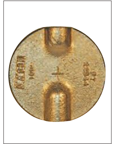
By Comparison – Flattened disc/boss areas of vertical disc design
