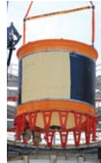
Figure 2: All-composite tank being tested at MSFC.
