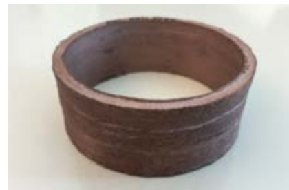
Figure 2: Combustion chamber liner ring (2.5 in inner diameter, 2.75 in outer diameter, 1 ft long) made from NARloy-Z-Cu-D composite.
