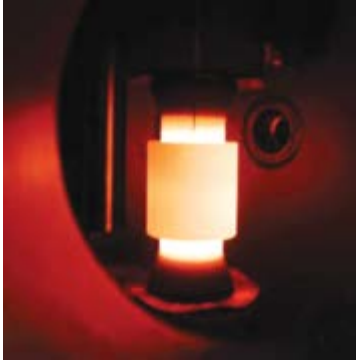
Figure 3: Sintering at high temperature using FAST at Applied Research Laboratory, Pennsylvania State University.
