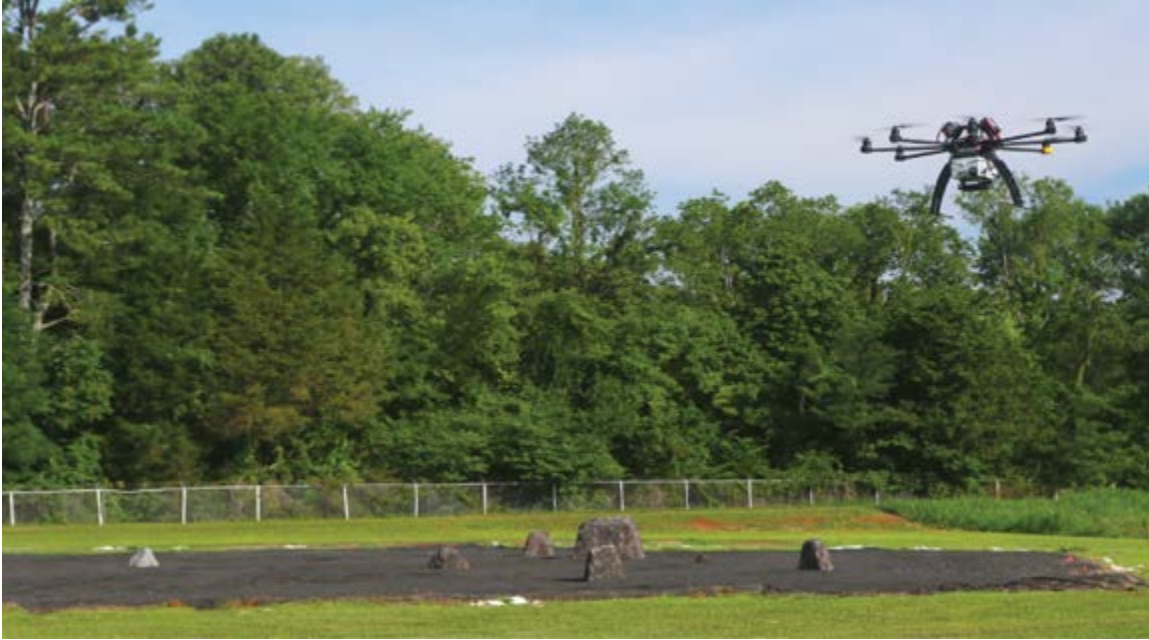
Octocopter flying over the terrain field carrying the radar.
