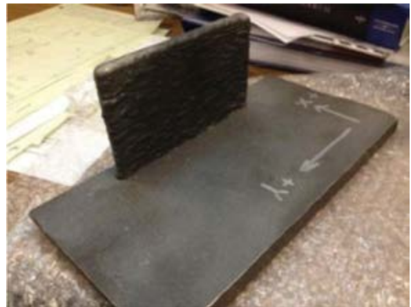
Figure 2: Typical MDDM Inconel® 718 build-up.
