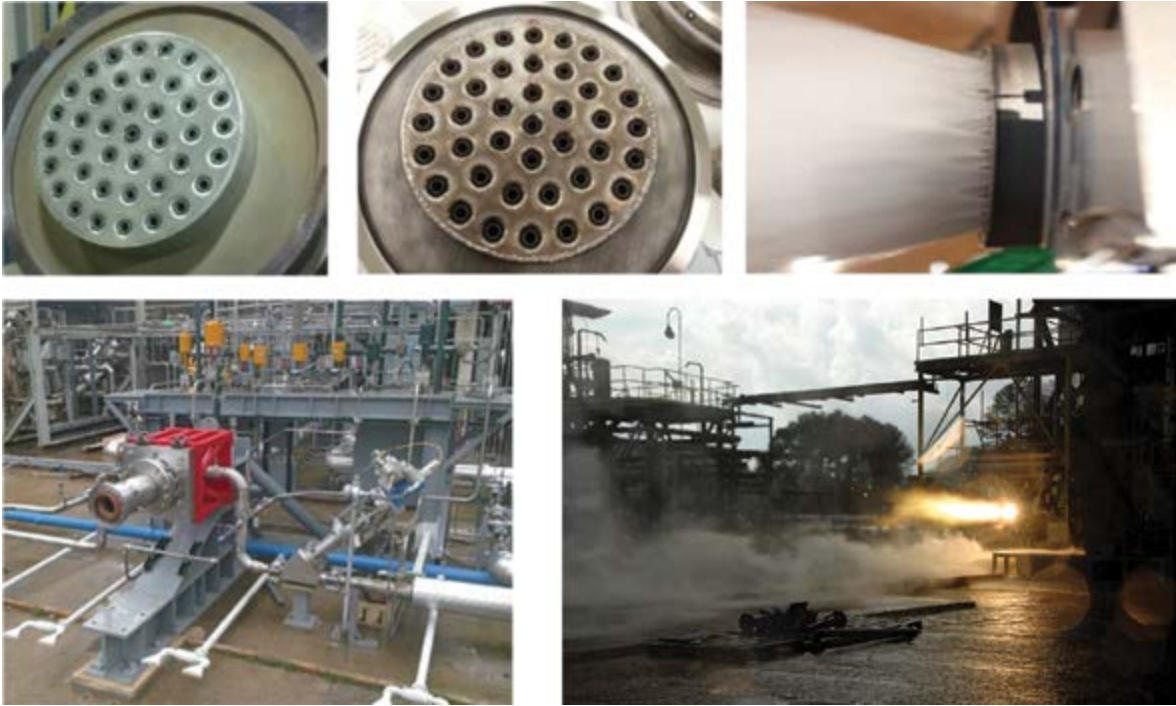
Figure 2: Water flow and hot-fire testing of two liquid oxygen/hydrogen SLM injectors.
