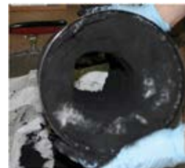
Figure 2: High-density carbon product containing dispersed iron catalyst.
