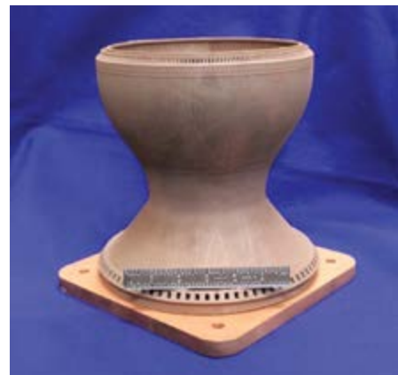
Throat section of combustion chamber fabricated utilizing SLM of high-strength copper alloy powder.
