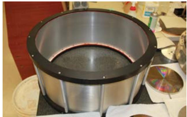
Figure 3: Full-shell polishing mount developed for the project.
