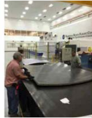
Removing cured panel from tool.
