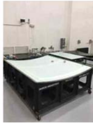
Vacuum bagged ready for cure.
