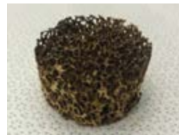
Figure 5: Iron coated on copper substrate using an ionic liquid.
