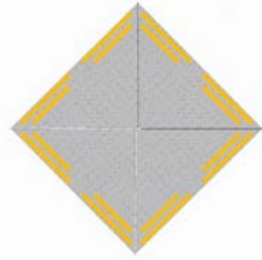
Figure 1: Conceptual render of reflective control devices along the edge of a solar sail (Source: NASA).
