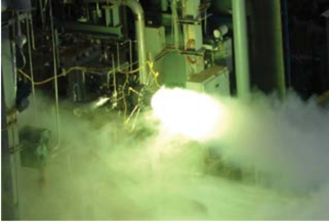
Figure 1: Oxygen-rich/RP-1 preburner testing at MSFC.
