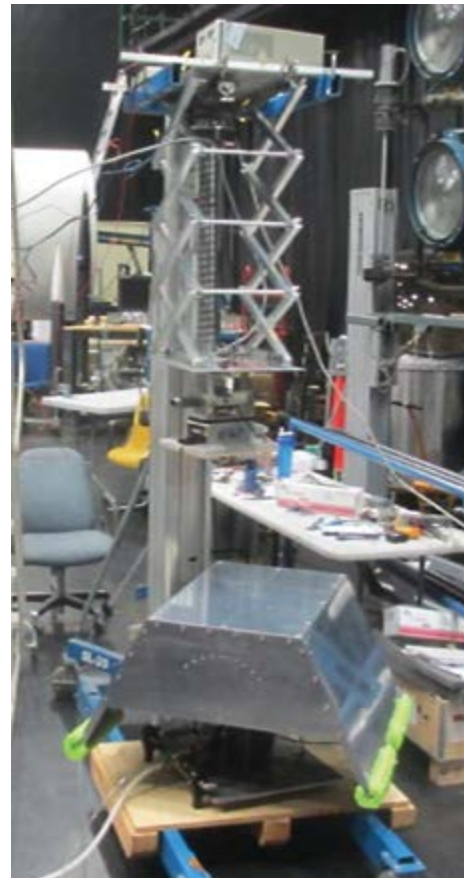
Intern-assembled retractable ES capture boom.
