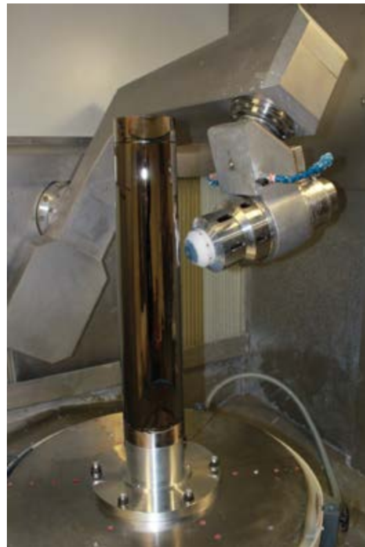
Figure 1: Computer-controlled polishing machine with the mandrel used for the validation of the developed polishing techniques installed.
