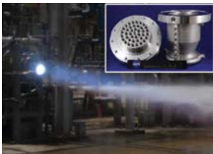
Figure 6: LOX/LCH 4 regenerative cool chamber hot-fire test.
