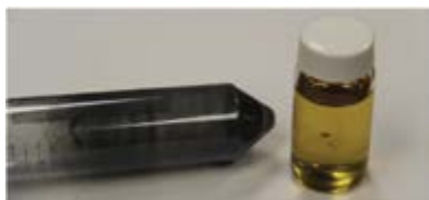
Figure 4: Carbon remaining after ionic liquid extraction (left) and ionic liquid containing iron (right).
