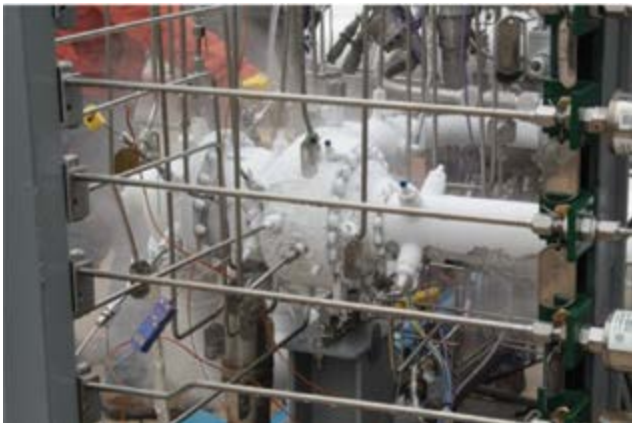
Figure 1: Turbopump LCH 4 chill testing.
