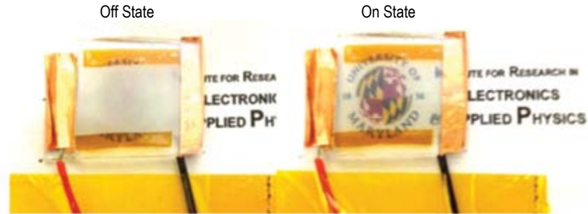
Figure 2: A functioning prototype of The University of Maryland reflective control devices. The material becomes transmissive when a voltage is applied, allowing photons to pass through in the on state (Source: The University of Maryland).
