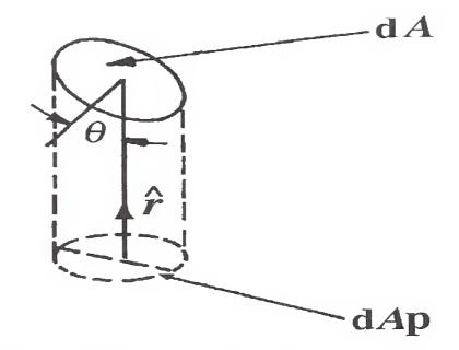
Figure 1. Illustration of the projected area.
