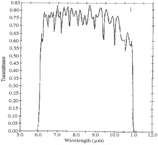
Figure 8. Typical bandpass interference filter transmittance.
