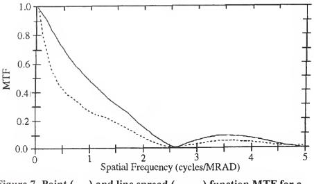
Figure 7. Point (----) and line spread ( \_\_\_\_\_ ) function MTF for a sensor.
