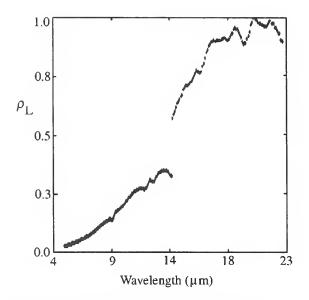
Figure 13. Relative spectral response  $\rho_{\rm L}(\lambda)$  or "instrument function" for the point-source absolute irradiance calibration.
