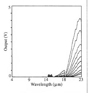
Figure 14. Scans obtained for the extended-area source absolute responsivity calibration.
