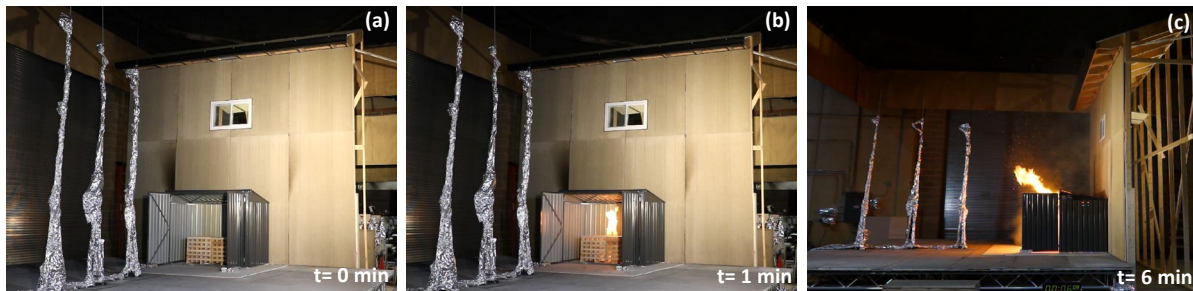
Fig. 83. Photographs captured from videos recorded by (a), (b) Camera #2, and (c) Camera #3, show steel Closet with low fuel loading, ignition of cribs, and flames coming out of the Closet in test 1B-SCI0-0.
