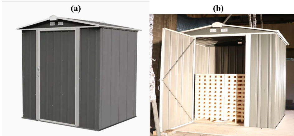
Fig. 40. Photograph of (a) steel Very Small shed (b) with high fuel loading of six 1-A cribs. Test 1B-SVSh0.
