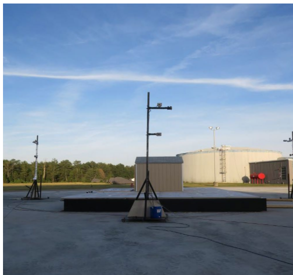
Fig. 121. Photograph showing experimental setup for outdoor free shed burn testing at the IBHS test facility. The photograph shows a shed on the weighing platform and the heat flux gauge rigs.
