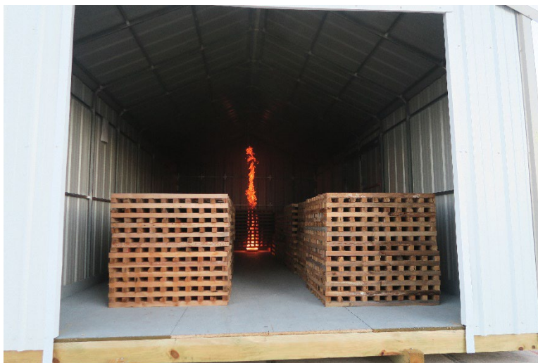
Fig. 125. An example of an ignition method using 300 mL of heptane in an aluminum pan placed underneath the back-middle crib.
