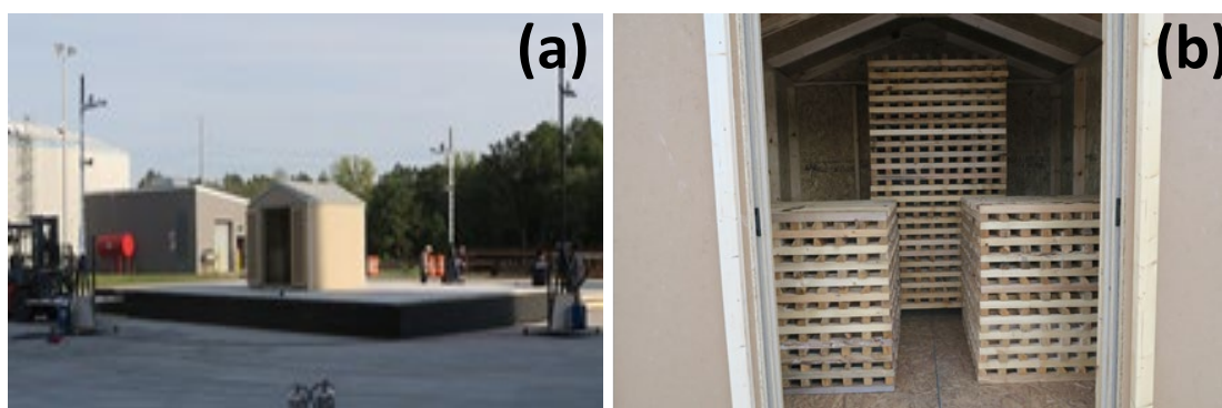
Fig. 126. Photographs of experimental setup showing (a) wood medium shed (b) with high fuel loading of four 6-A cribs.
