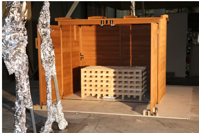
Fig. 45. Photograph of wood Closet with low fuel loading of two 1-A cribs. Test 1B-WC10.
