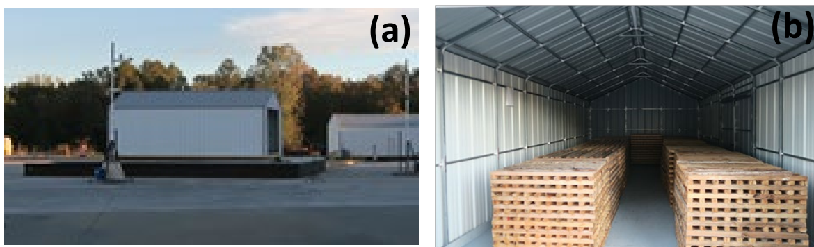
Fig. 145. Photograph of (a) steel Very Large shed setup with (b) high fuel loading of 15 wood cribs.
