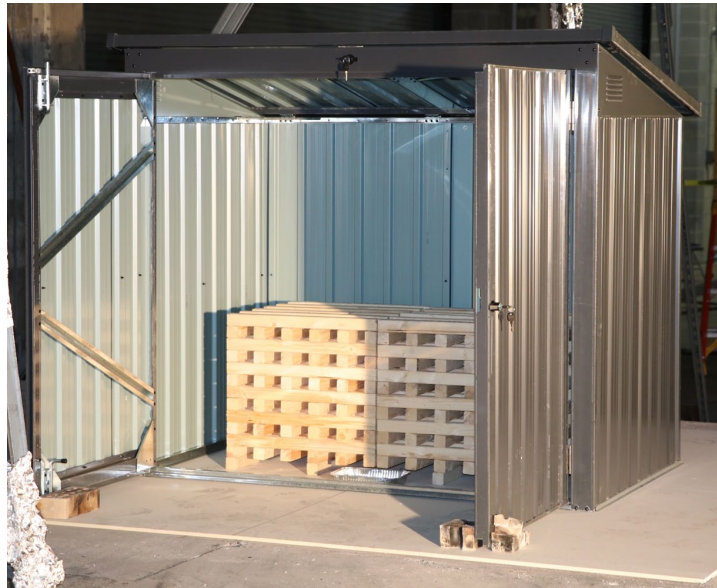
Fig. 55. Photograph of steel Closet with low fuel loading of two 1-A cribs. Test 1B-SCI0.
