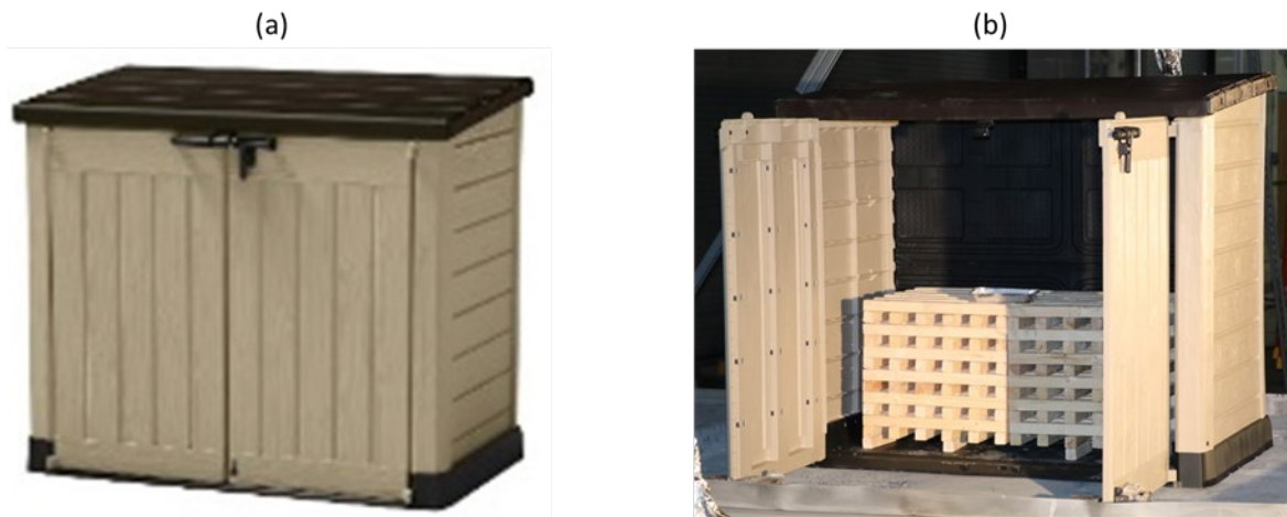
Fig. 50. Photograph of (a) plastic Closet (b) with low fuel loading of two 1-A cribs. Test 1B-PCI0.
