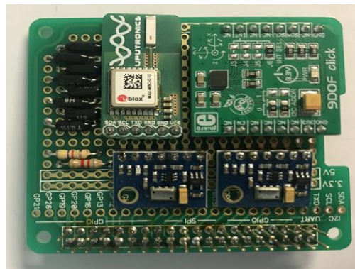
Figure 6. Prototyping HAT used for the equipment and OBC interconnections.
