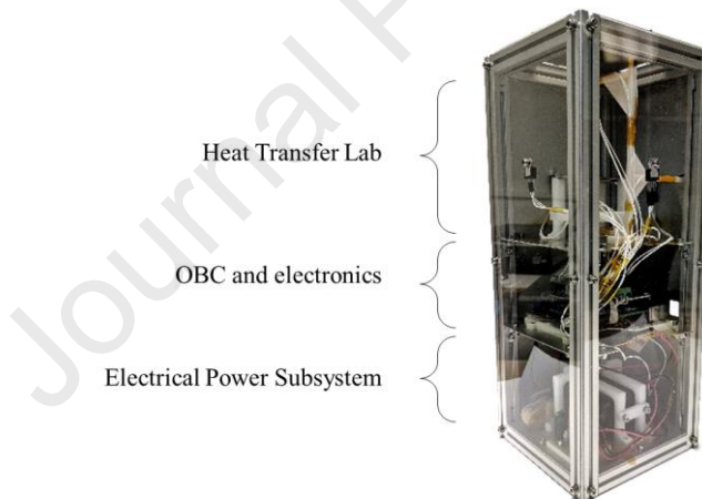
Figure 2. TASEC-Lab structural configuration.
