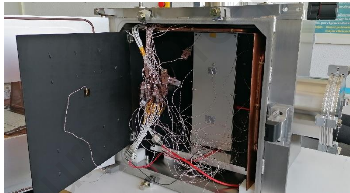
Figure 19. Opened TVAC chamber with TASEC-Lab and thermocouples connections.
