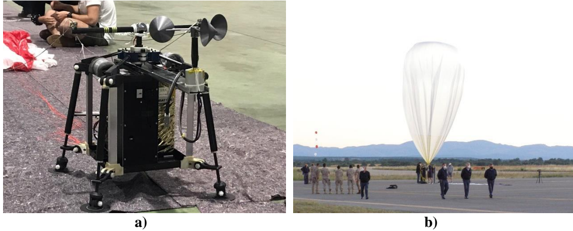
Figure 21. a) Gondola final configuration during the parachute integration and b) balloon film during the inflation.
