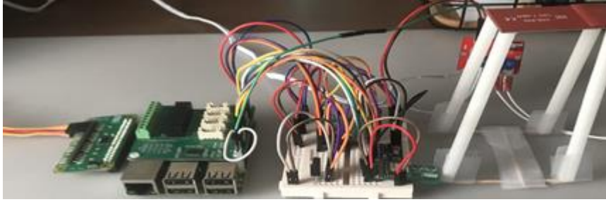
Figure 14. Prototyping model of TASEC-Lab used for software testing.
