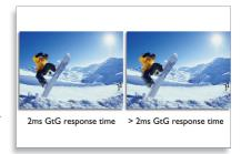
SmartResponse is a exclusive Philips overdrive technology that when turned on, automatically adjusts response times to specific application requirements like gaming and movies which require faster response times in order to produce judder, time-lag and ghost image free images
