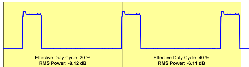
Figure 10 – "Wrong" RMS detection of pulsed signals
