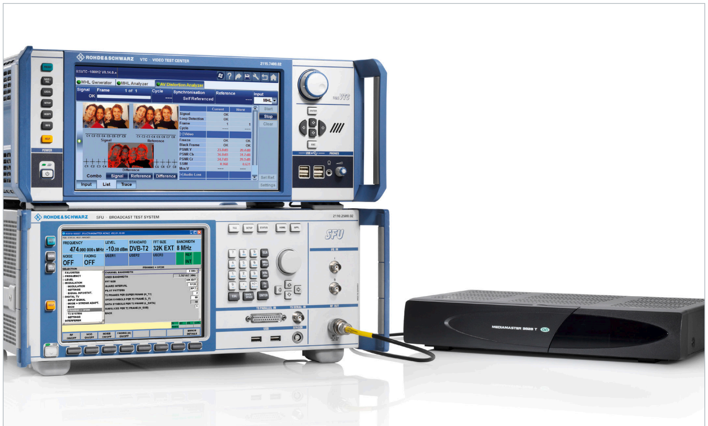
The R&S®VTC and the R&S®SFU for testing a set-top box
