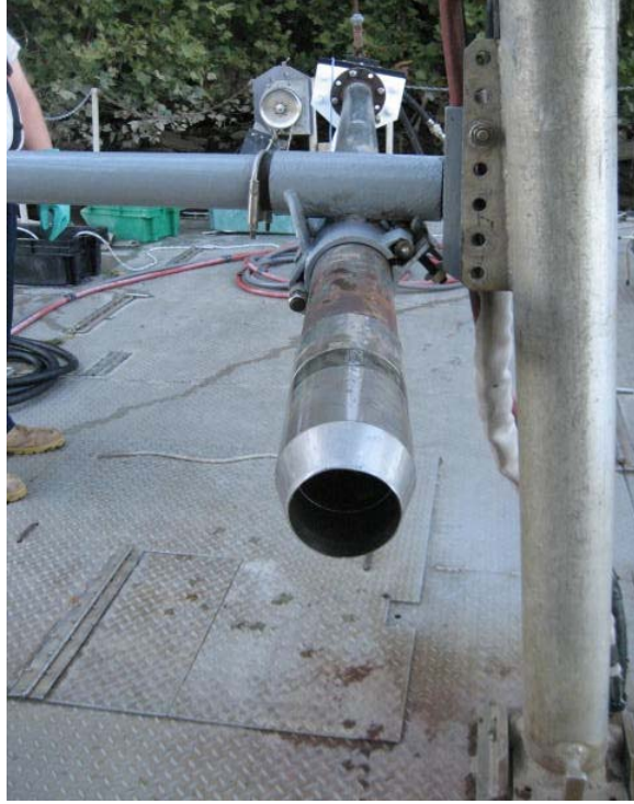
Photo 1 - Vibracore Core Barrel Sampler
