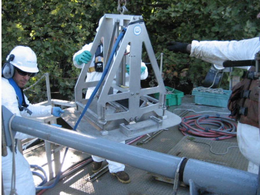
Photo 7 – Lowering Powergrab sampler
