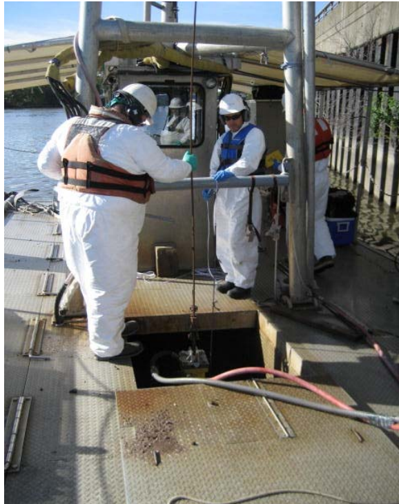
Photo 2: Vibracoring at SSP2 location 13B-0547
