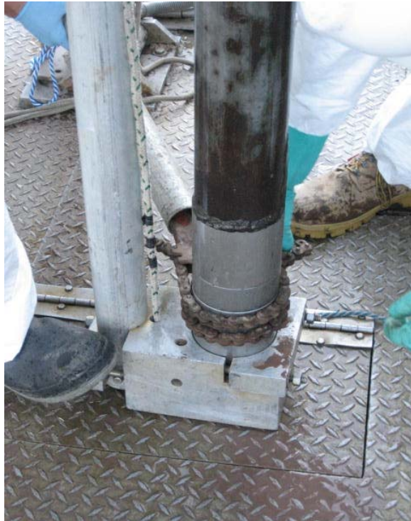
Photo 4 - Removing shoe from core barrel to extrude sample liner
