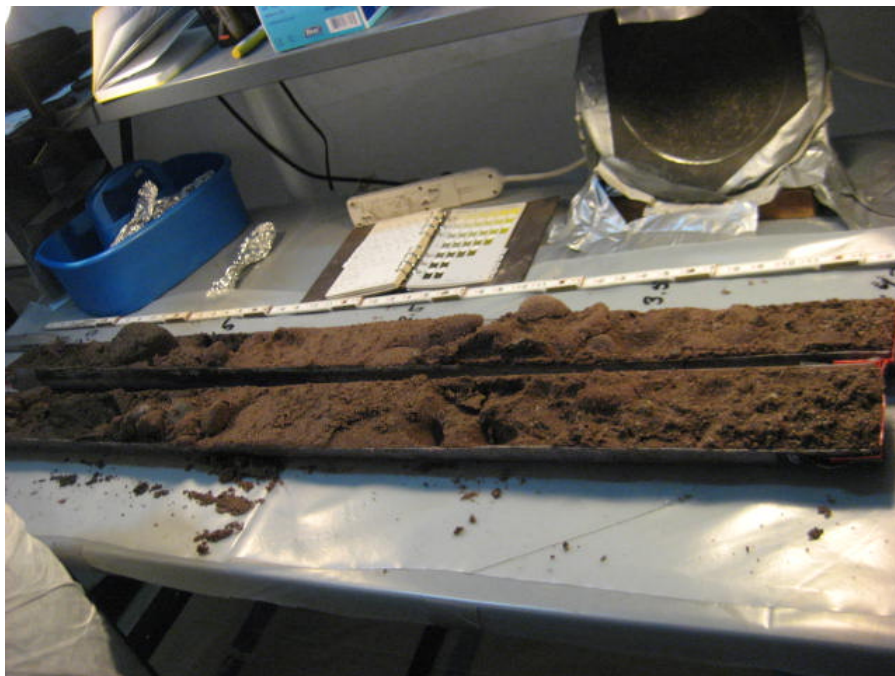
Photo 14 - Sample core opened to perform geologic characterization
