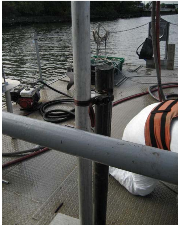
Photo 6 – Core liner was cut into 5' sections to enable safe handling during transportation
