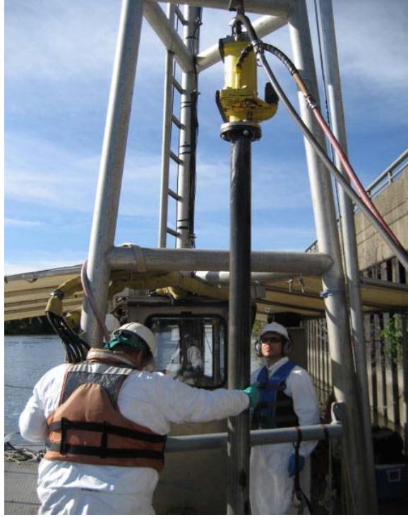
Photo 3 – Pulling up core barrel at SSP2 location 13B-0547
