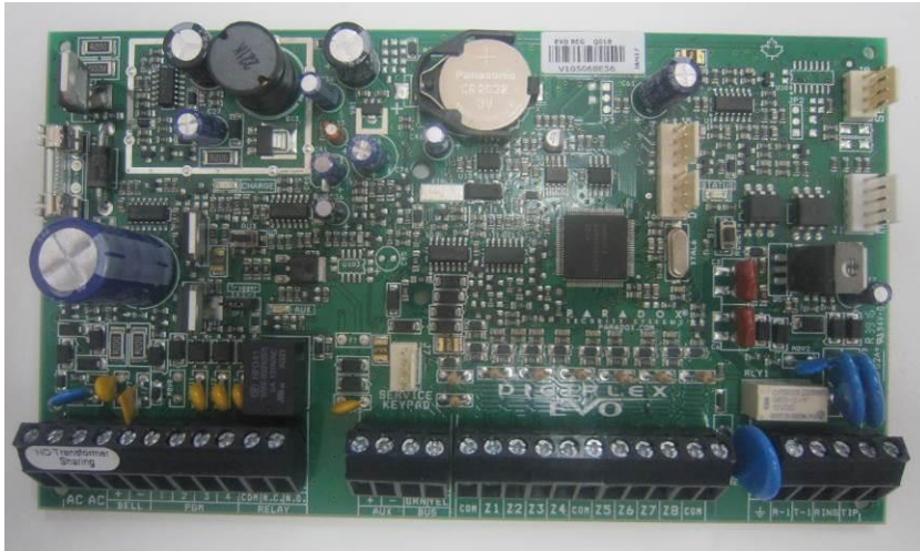
Photograph 5.1.2, 5.1.3 – EVO192 PCB view
