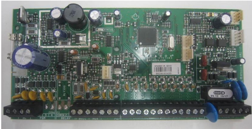
Photograph 5.1.8, 5.1.9 – SP6000 PCB view
