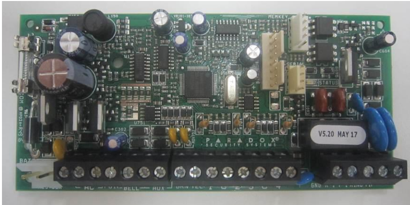
Photograph 5.1.4, 5.1.5 – SP4000 PCB view
