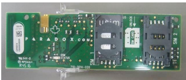
Photograph 5.1.17, 5.1.18 – GPRS module for MG6250 view
