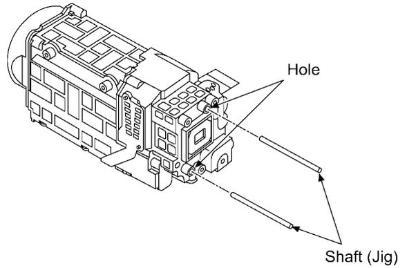
2. Insert the shafts through the holes on the MOS fixing angle, fix the position of the MOS(1).
