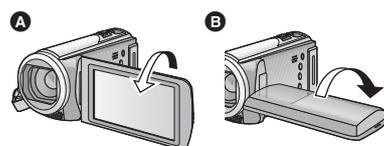
• It can rotate up to 180° **A** towards the lens or 90° **B** towards the opposite direction.
