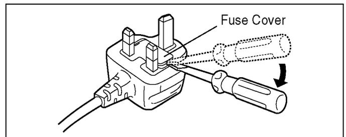
2. Replace the fuse and attach the Fuse cover.
