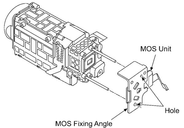
3. Tighten 3 screws and fix the MOS unit.
