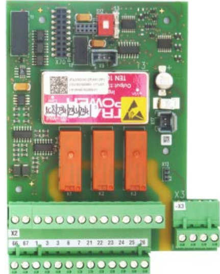
Peripheral board DI/DO
