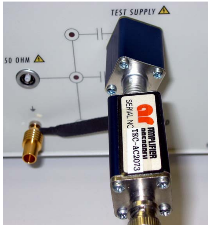
FIGURE 2: COAXIAL ADAPTER FOR BURST PULSE OBSERVATION
